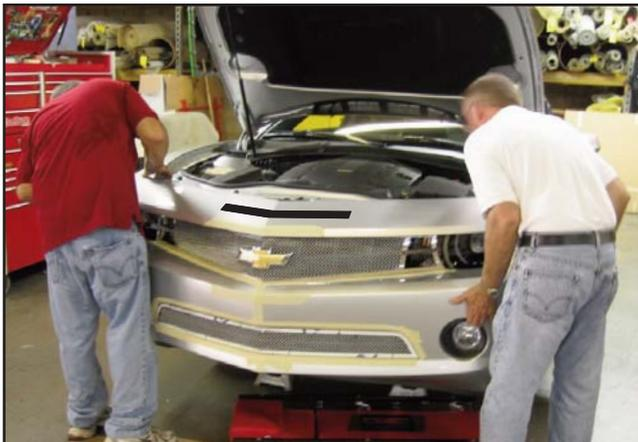
50. With the help of an assistant, realign the bumper cover back onto the vehicle, making sure the alignment pins line up with the holes in the front fenders. Reverse the removal procedure to reinstall the front bumper cover back onto the vehicle. Once the bumper cover is secure, remove the protective masking tape (not shown).
