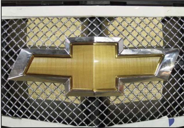
42. Align the emblem assembly onto the mesh grille, making sure the mounting studs fit through the holes drilled in *Step 30*.
