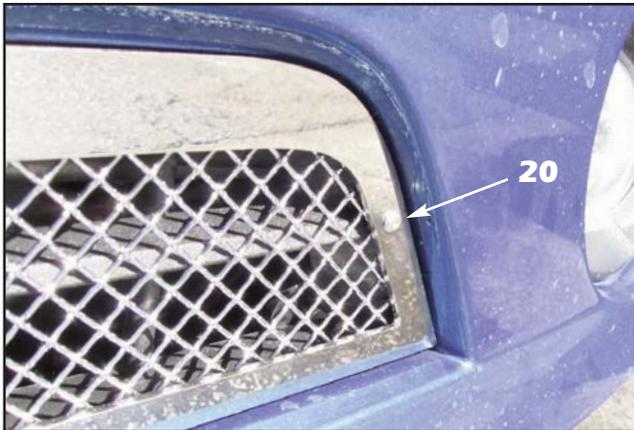
20. Use a 1/16" drill bit to drill through the holes in the lower surround and install the supplied #6 x 3/4" torx pin head screws (RS shown, SS similar).
