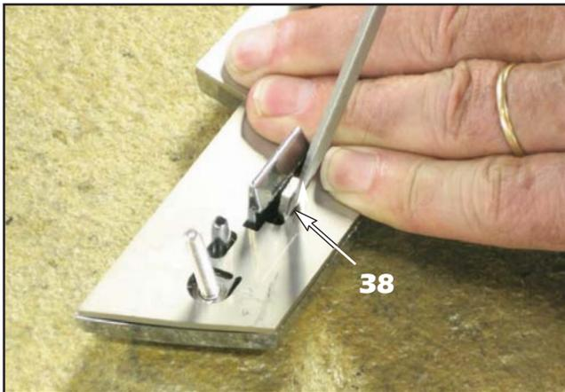
38. Using a small flat blade screwdriver, fit the tip down into the **small slot** cut into the **tab** (as shown).
