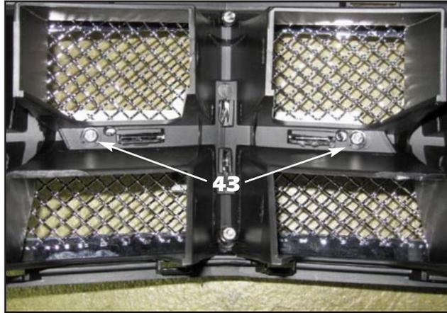
43. Install the supplied **#8-32 ESNA half nuts** and **small black plastic washers** to secure the emblem to the mesh grille.
