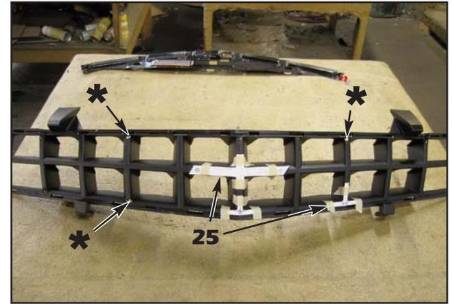
25. Cut out the supplied **templates** and tape them into place as shown. The **outer hole location template** is used at all additional areas indicated in the above picture with an **asterick \***.
