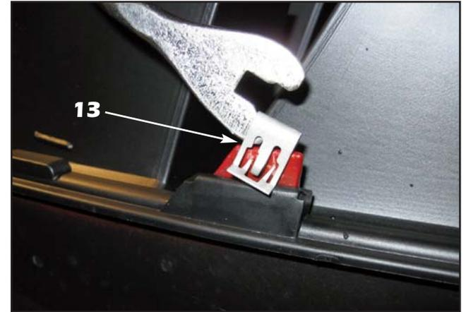
**13.** Use a small flat blade screwdriver to remove the metal retaining clips underneath the factory upper grille insert. A door panel clip removal tool (shown) works as well.
