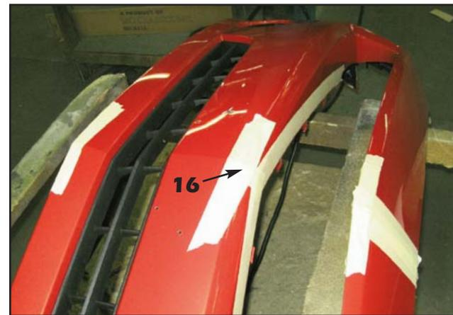
**16.** Apply additional layers of masking tape to the bumper cover once the front tag bracket has been removed.
