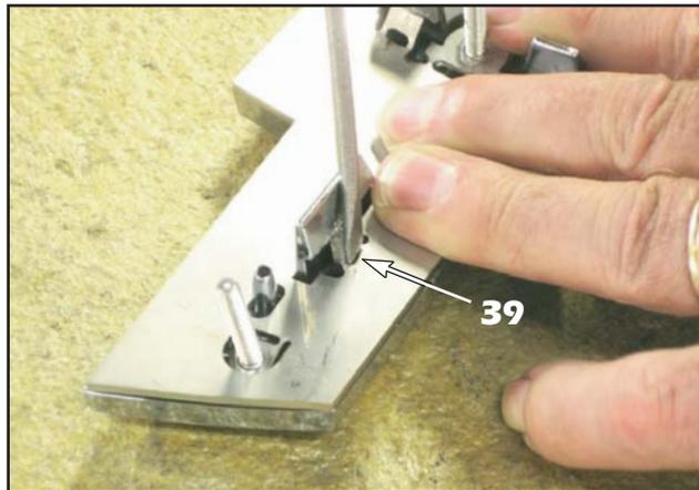
39. Bend the **retaining tabs** towards the factory mounting tabs until they hook underneath, locking the emblem to the **mounting plate**.
