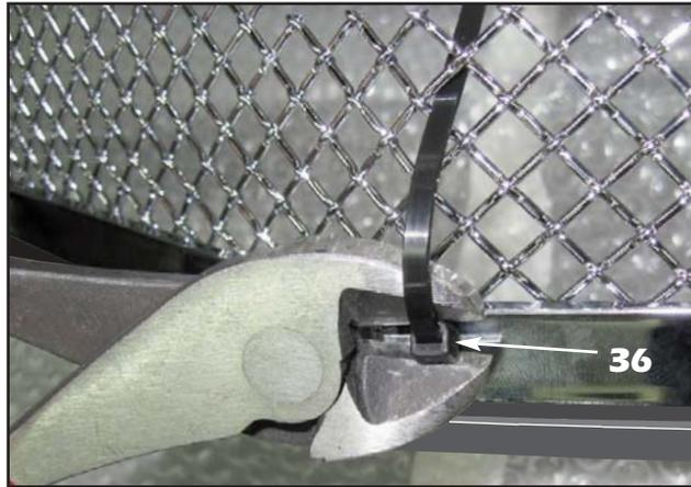
36. Turn the bumper cover assembly over and make sure that the mesh does not protrude past the edges of the surround, and that the surround does not overlap the mounting channel of the factory grille insert. If it overlaps, you will not be able properly install the grille back into the bumper cover. **Shift the mesh or surround as necessary. Snug the ESNA half nuts (do not completely tighten at this time), then cut off the black cable ties.**
