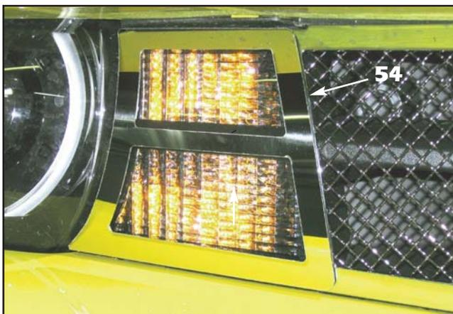
54. Peel off the protective liner from the stainless steel overlay and use a mild solvent to remove any glue residue. Use alcohol or glass cleaner to remove any solvent residue.
