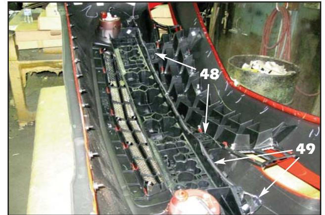
48. Once the upper and lower grilles are in place, reinstall the plastic bumper reinforcement by snapping it over the bosses on the factory portion of the upper grille assembly.
