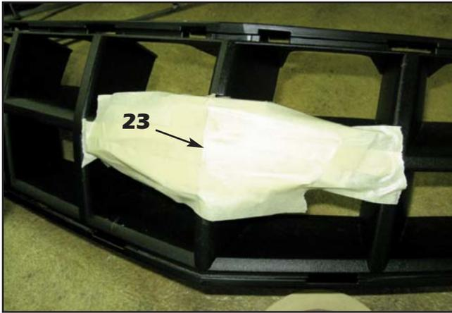
23. Apply layers of masking tape to the grille emblems (bow tie emblem shown, do the same to the "RS" emblem if equipped).
