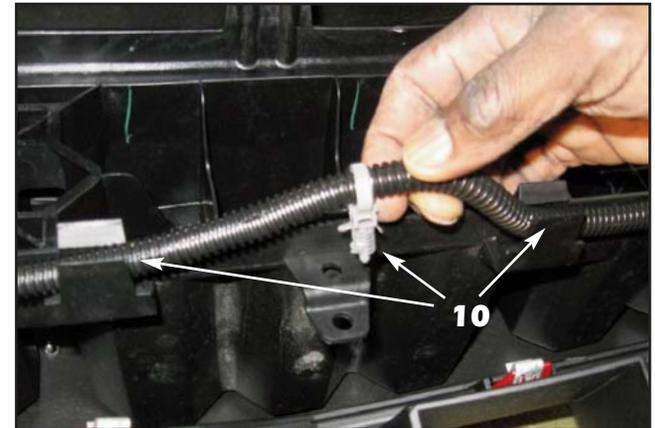
10. Turn the bumper cover over and remove the wire harness from the plastic front bumper support.
