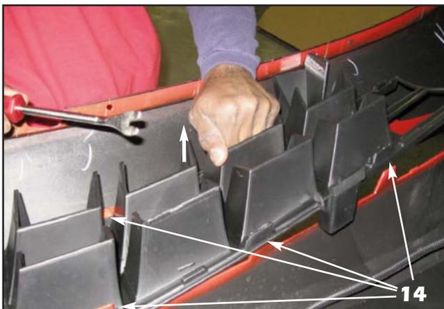
**14.** Remove the factory grille insert by using a small flat blade screwdriver to pry out on the factory insert to clear the mounting tabs on the bumper cover, then pull the factory grille insert out from the back.
