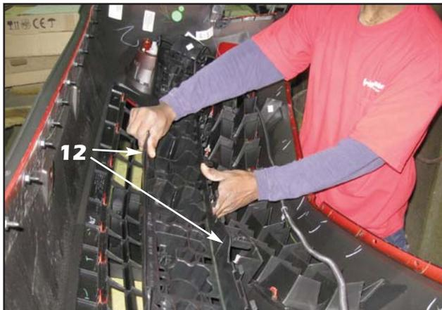
**12.** Unclip and remove the plastic bumper reinforcement from the back of the bumper cover.
