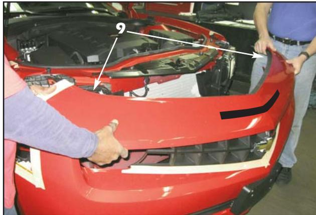
9. With the help of an assistant, place the bumper cover onto a clean, flat work area, face up for the following procedures.
