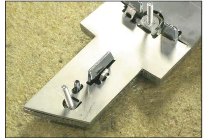
37. Align the **emblem mounting plate** over the back of the factory grille emblem, making sure all the factory mounting tabs pass through the slots in the **mounting plate**.
