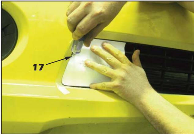
17. Cut out and align the **lower hole location template** onto the lower grille in the bumper cover opening and use masking tape to hold it in place. Use an awl or similar pointed tool to mark the hole location onto the plastic grille (as shown). Untape the **template**, flip it over and mark the opposite side.
