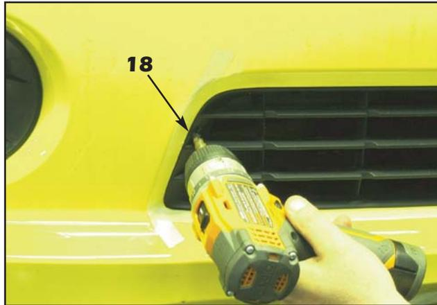
18. Use a 5/16" drill bit to drill through the marks made in the plastic lower grille prior to grille alignment.
