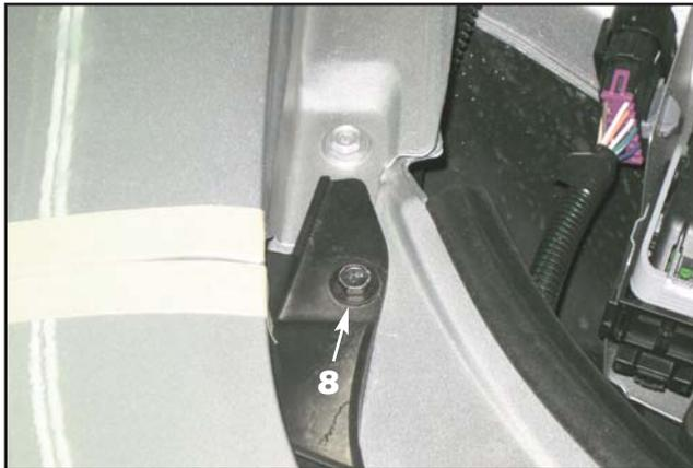
8. With the help of an assistant, remove the top outer 10mm hex bolts retaining the bumper cover to the front fenders. Do not let the bumper cover shift or move until you are ready to pull the bumper cover free from the front fenders.
