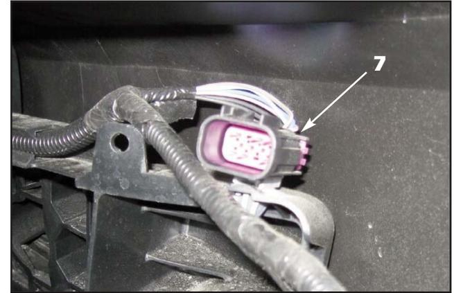
7. Unplug the main electrical harness at the connector located on the passenger side underneath the headlight assembly by pushing down on the plug clip to release.
