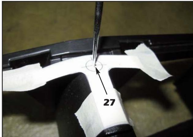
27. Once the lower center hole location is marked, remove the template, turn it upside down and tape it to the top of the grille, making sure the top center is flush with the edge of the channel. Mark the hole location once taped into place.
