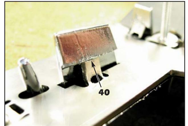
40. Close up of the **retaining tab** properly bent to engage the factory mounting tab, keeping the emblem tight against the **mounting plate**.
