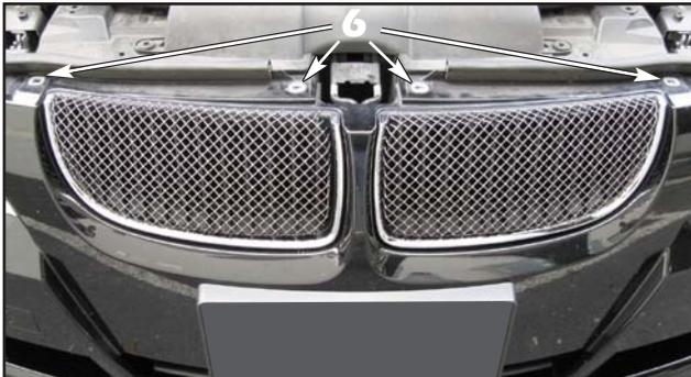
6. Align the assembled grille sections back into the bumper cover, making sure that they clip back into the factory mounting slots.
