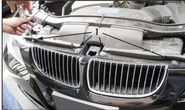
1. Open the hood and remove the four (4) Torx T-25 screws from across the top of the factory grille.
