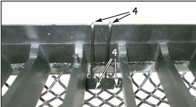
3. Align the mesh sections over the factory grille sections.
