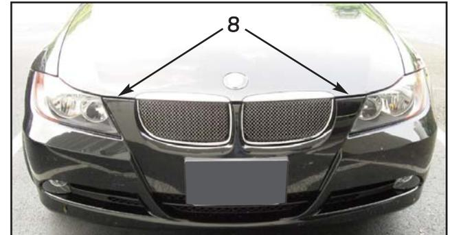
8. Close the hood and check for proper bumper cover to hood alignment. Adjust accordingly, then open the hood and tighten the torx screws to finish.
