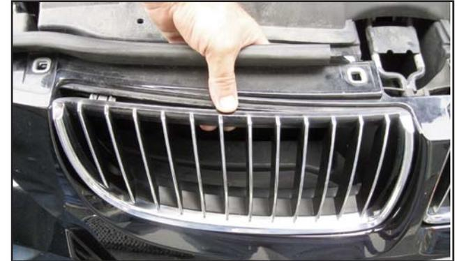
2. Pull forward on the top of the bumper cover and push up on the centers of the upper mounting tabs and push the grille sections forward to remove them from the bumper cover. **Note:** If the factory grille have chrome verticle bars, scuff the chrome verticle bars and paint them flat black.
