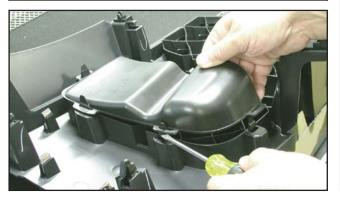
Place the grille onto a clean work surface and remove the left and right air deflectors from the back fo the upper grille by prying out with a flat blade screw driver.
