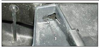
1. Open the hood use a long flat blade screw driver to rotate the exposed mounting clips that retain the upper grille. Turn them approx. 1/8 of a turn and the clips will release.
