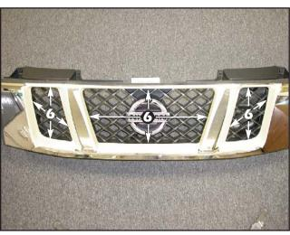
Apply protective masking tape to the factory upper grille as shown. This will help protect the factory grille finish while installing the stainless steel grille sections.
