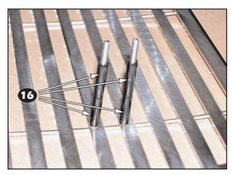
16. For "Q" grille: Install two (2) black silicone sleeves onto each mounting stud (trim the ends off with cutters or a razor blade). Install the black trim guard around the edge of the grille with the seam at the top.
