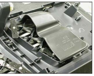
13. Reinstall the factory air defelctors back onto the assembled upper grille by snapping them back into place.
