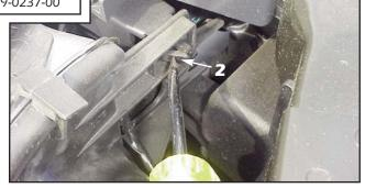
2. The top two mounting clips on each side that retain the upper grille can be release by pushing in on the side of the clip and pulling straight out.
