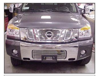
**22**. Reinstall the upper grille assembly to finish the installation.
