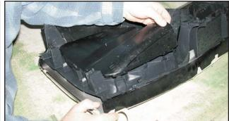
3. Place the grille onto a clean work surface and remove the left and right air deflectors from the back fo the upper grille by pulling straight out.
