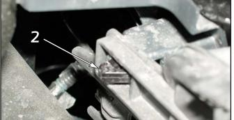
2. The top two mounting clips on each side that retain the upper grille can be release by pushing in on the side of the clip and pulling straight out. Remove all clips from the radiator support panel.
