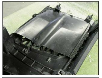
11. Reinstall the factory air deflectors back onto the assembled upper grille by snapping them back into place.
