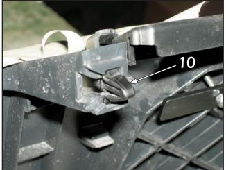
**10**. Remove the factory clips in the radiator support panel and reinstall them into the upper grille.
