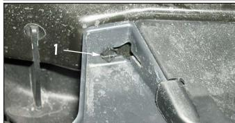
1. Open the hood use a long flat blade screw driver to rotate the exposed mounting clips that retain the upper grille. Turn them approx. 1/8 of a turn and the clips will release.
