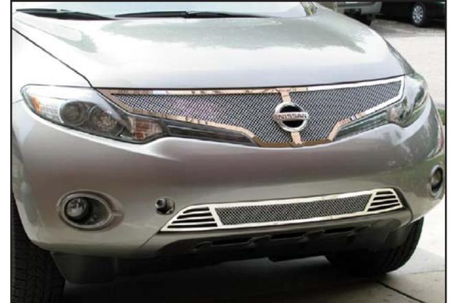
31. Remove the protective coverings from the grille sections and thoroughly clean the grille once you are finished the installation. A mild solvent followed by glass cleaner works very well. **CAUTION! Be careful while cleaning the edges of the grille frame as the edges of the stainless steel can be very sharp.**
