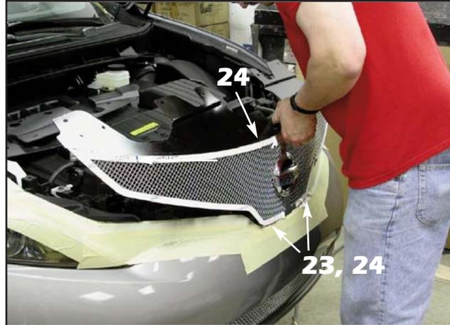
23. Remove any masking tape that could get caught underneath the center portion of the grille at the mounting pin locations.
