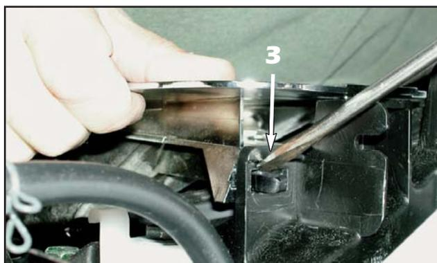
3. Pull the grille out at the top, use a flat blade screw driver to push down on the top of the clip and pull the grille straight out to release the top outer clips from the mounting slots (one each side).
