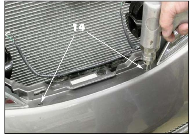
**14.** Use a 1/8" drill bit to drill through the marks made in the previous step, then use the drill to connect the holes making a mounting slot. This will allow for slight left to right adjustments during the grille installation.
