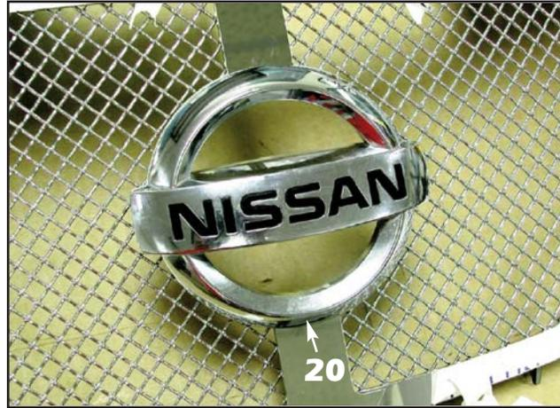
20. Align the factory emblem onto the assembled grille, making sure all factory mounting tabs pass through the slots in the emblem center bar.
