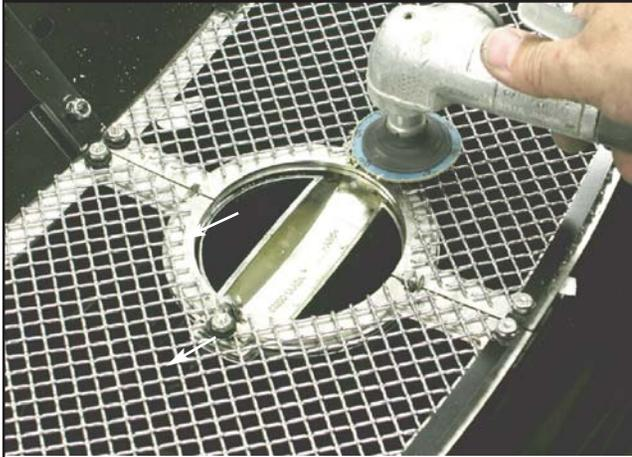
22. Use a disc grinder or cutters to shorten the factory mounting clips on the emblem. This will keep them from being visible when the grille is installed on the vehicle.
