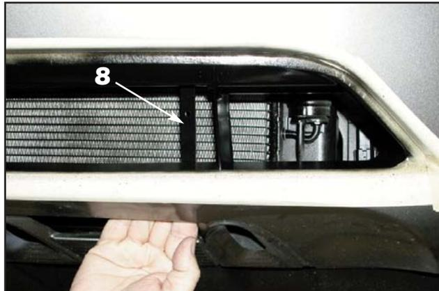
8. From underneath the vehicle, insert the lower grille mounting brackets between the metal bumper reinforcement and the styrofoam filler approximately 1" inside the outer vehicle dividers (on each side). The tension of the angle the brackets rest against the metal bumper and the bumper cover will hold the brackets in place while you align the lower mesh grille into the opening.
