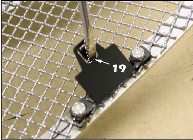
19. Use a flat blade screwdriver to bend the center of the mounting brackets up towards the mesh sections of the grille. Make sure you bend it up enough that the bottom of the tabs is just above the top surface of the bracket (bend it up at least the thickness of the metal).
