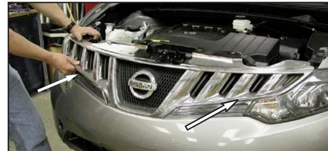
4. Pull the grille out so that the outer clips from the previous step clear the mounting slot, then lift up slightly on the grille in order to get your hand between the bottom of the grille and the top of the light (where shown). Give a quick pull straight out to release the next inboard mounting clips (one each side at arrow locations), the clips are not easily accessible with tools, so the mounting clips might break during removal but they are not reused.
