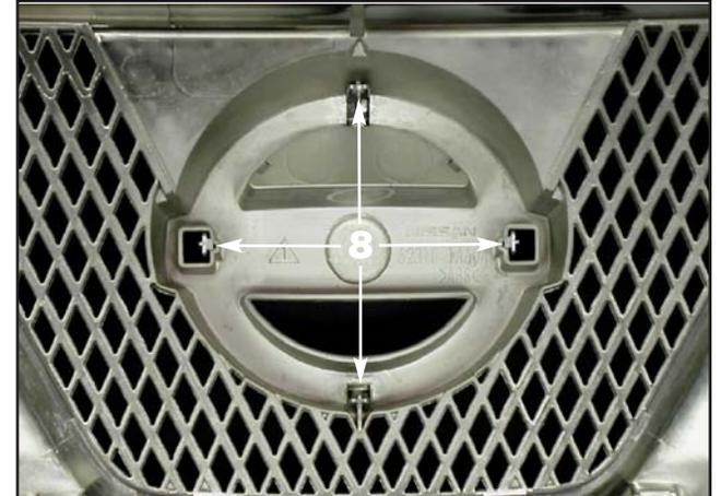
8. Unclip the factory emblem from the O.E. grille for installation onto the E&G Mesh grille.
