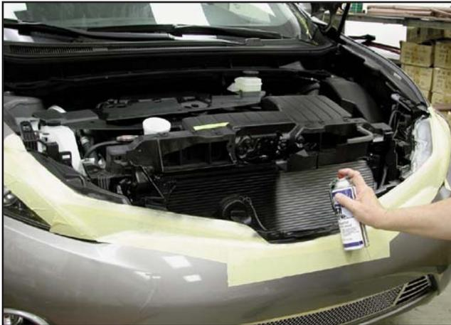
**15.** E&G recommends that everything visible in the grille opening be painted flat or semi gloss black. You will see through the E&G grille once it is installed and blacking out the radiator, bumper reinforcement, lower mounting holes on light colored vehicles, etc. will make for a professional appearing "factory" installation.
