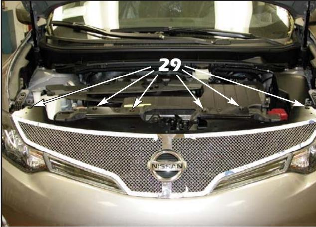
29. Reinstall the push fasteners removed in **Step 2** to secure the top plate to the radiator support panel.
