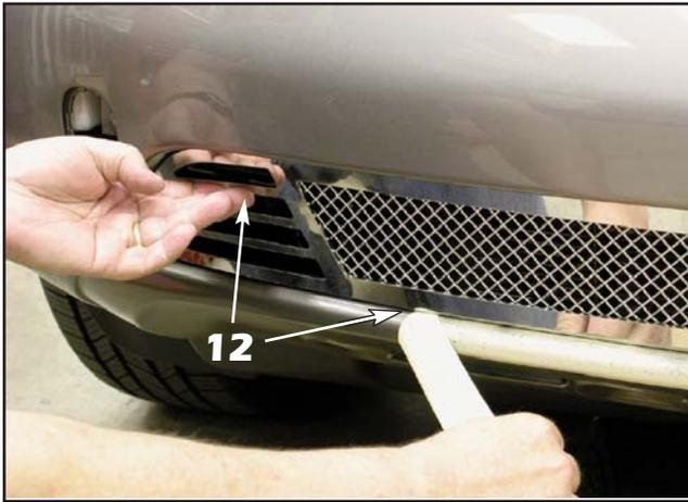
**12.** Lift up on the lower grille and pull off the masking tape. Pull the tape back over itself to minimize the tape braking and getting caught behind the grille.
