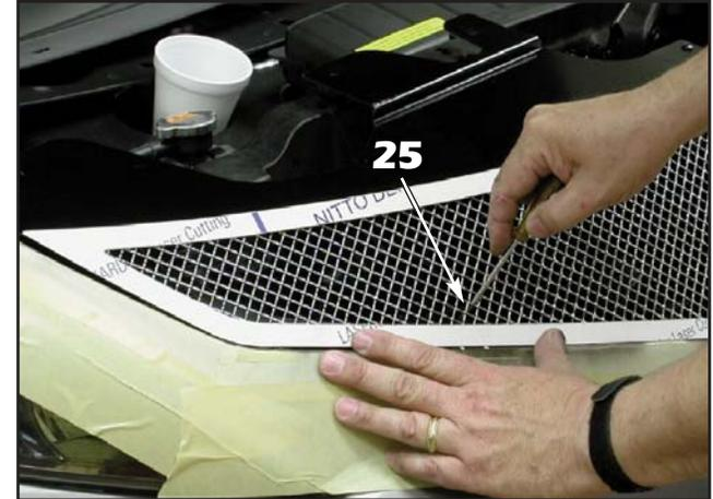
25. Pull out on the grille and push down until the mounting brackets line up with the mounting slot above the lense. Use a small flat blade screw driver to push down on the center of tab while pushing back onto the bottom of the grille until the tab clips into the mounting slot.
