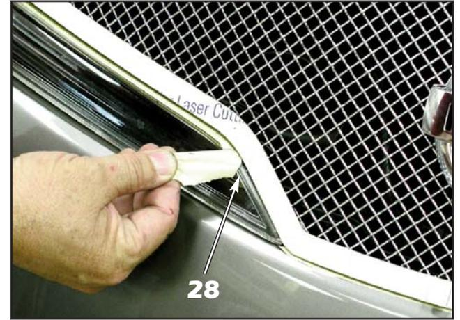
28. Once both mounting brackets are secured, lift up slightly on the grille and remove all protective masking tape from the front of the bumper cover and headlamp lenses.
