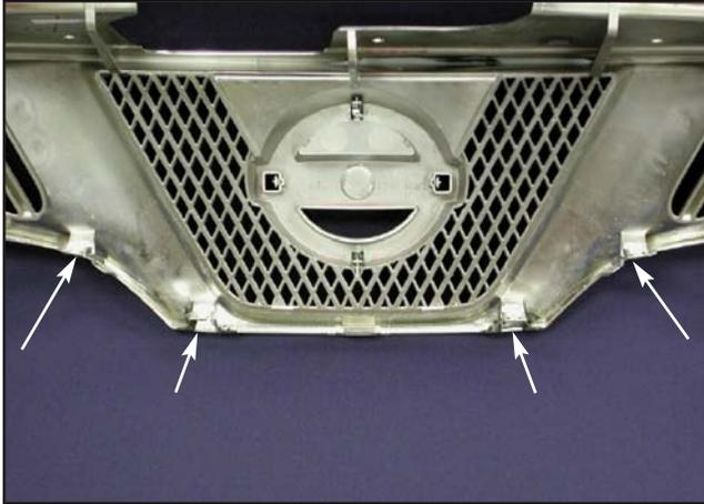
5. The photo above shows the locations of the four lower mounting clips. The grille is shown removed from the vehicle in order to show the locations as they are difficult to photograph with the grille still attached to the mounting brackets.
