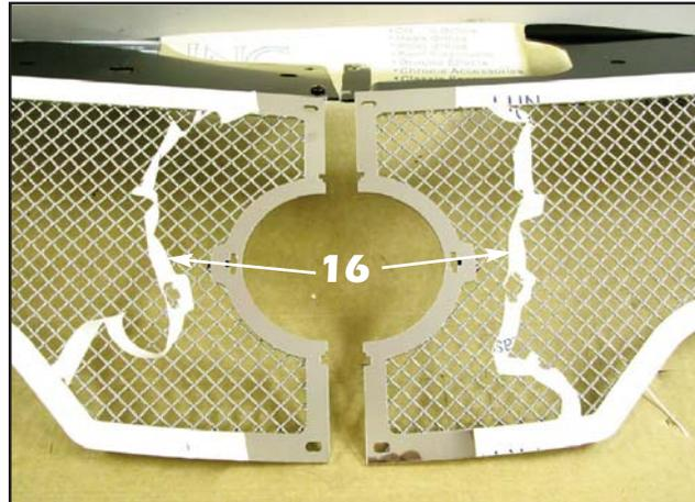
**16.** Lay the two pre-assembled mesh grille sections onto a clean work area and peel back the protective liner from the face of the grille sections in preparation for assembly.
