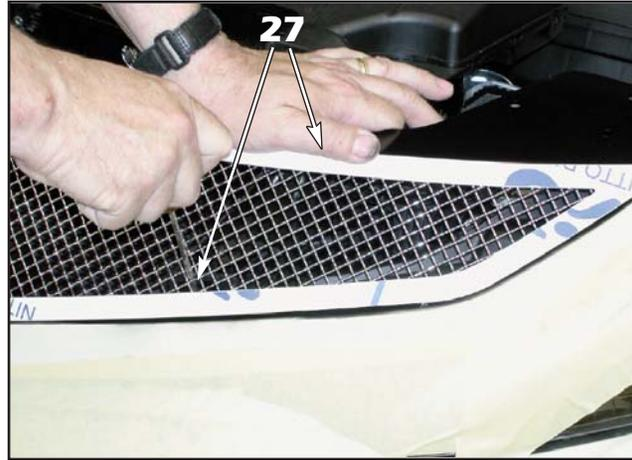
27. Use a small flat blade screw driver to push down on the center of tab while pushing down onto the top of the grille until the tab clips into the mounting slot.
