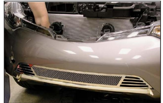
9. Remove the masking tape from the sides and the top of the lower grille opening.
