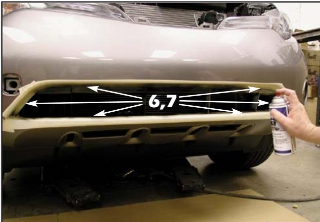
6. Using masking tape, tape up to the edges of the vertical supports and 1/4" inside the sides and top of the grille return edge.
