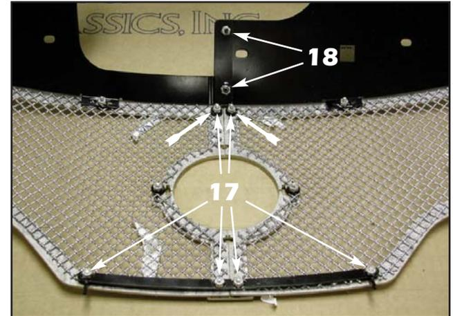
**17.** Assemble the two grille sections together using the emblem center bar, lower retainer w/ mounting pins, the small black plastic washers (where shown with bold arrows) and #8-32 ESNA half nuts.
