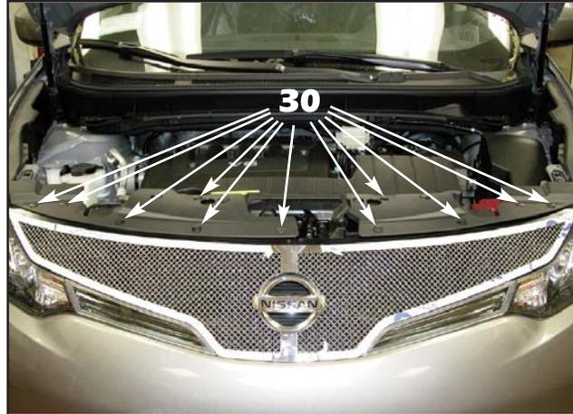
30. Reinstall the two factory plastic covers over the E&G top plate, reusing the factory push fasteners removed in **Step 1**.
