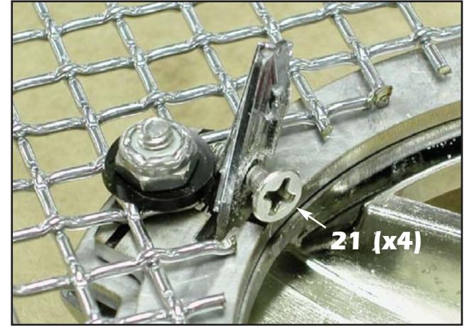
21. Turn the grille over and use a 3/32" drill bit to drill through all four (4) mounting tabs close to the surface of the grille and install the supplied #4 x 3/4" oval head phillips screws to secure the emblem to the mesh grille.
