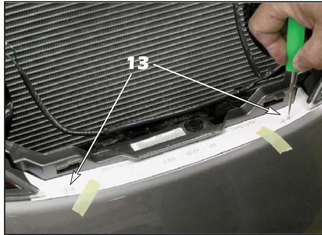
**13.** Cut out and align the supplied template onto the bumper cover between the clear plastic lenses. Use an awl or similar pointed tool to mark the hole locations onto the bumper cover.
