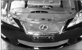
**39**. Reinstall the factory radiator support panel cover.
