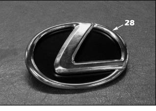
28. Peel off the tape backing, align the emblem onto the emblem mounting plate and press firmly to set the tape.
