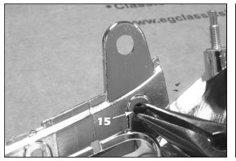
15. Remove the outer rubber moulding clips and reinsert them into the rubber moulding.
