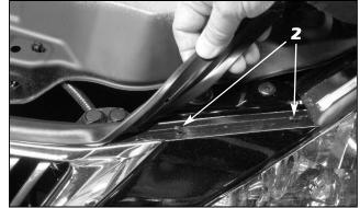
Unclip the factory weatherstrip from the bumper cover. You can pull and stretch the weatherstrip off of the mounting clips to release it.
