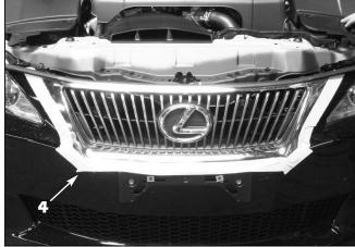
4. Apply masking tape to the perimeter of the grille (as shown) to protect the painted bumper cover during the following factory grille removal procedure.
