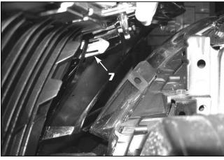
Once the screws are removed, squeeze the centers of the verticle mounting tabs in and pull the factory grille forward to clear the mounting slots in the bumper cover.
