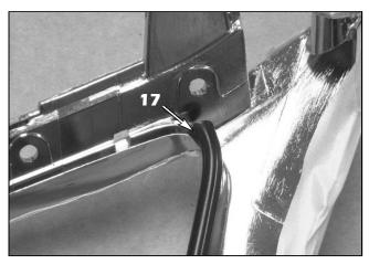
17. Begin the installation of the black edge guard at the upper radiused corners of the factory chrome surround (where shown). Make sure that the longer, tapered edge of the edge guard fits over the visible side of the factory chrome surround.
