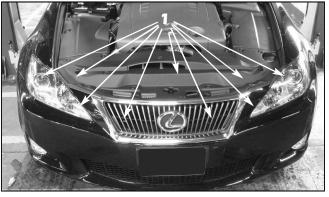
**1**. Open the hood and remove the plastic header panel cover by removing the plastic push fasteners with a small flat blade screw driver (push down on the center of the clip to release, not shown).
