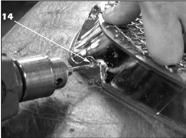
14. Use a 1/8" drill bit to create a small slot in the lower tabs located on the factory chrome frame. Make them wide enough for to install the .130" wide cable ties supplied with this kit.
