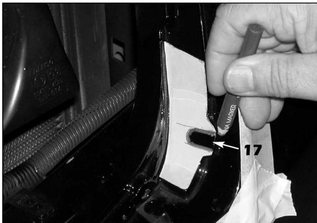
17. Cut out and align the supplied template where shown. Use a grease pencil to mark the notch in the template onto the bumper cover. Once marked, repeat on the opposite side of the grille opening.
