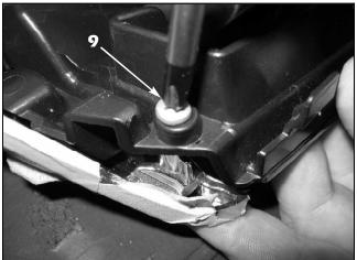
Remove the factory screws retaining the insert to the factory chrome surround.
