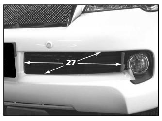
27. Apply masking tape to the edges of the lower grille openings to protect the paint during the following lower mesh grille installation procedure.
