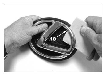
18. Use a plastic Squeegee to seperate the factory emblem from the base. Do not use a metal tool such as a screw driver or you will damage the edges of the emblem.
