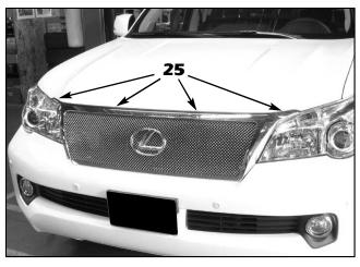
25. Align the assembled mesh grille into place and press down firmly to seat the lower retaining pins into the slots drilled in the bumper cover. Reinstall all applicable factory mounting hardware to secure the grille. Close the hood and check for proper depth alignment at the hood. You can adjust the grille in or out as needed.
