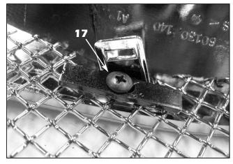
17. Align the supplied black rectangular mesh retainers along side of the factory mounting tabs located on the sides of the factory surround and use a 7/64" drill bit to drill through the center of the slot in the black rectangular mesh retainer. Install the retainer with the supplied #8 x 1/2" black truss head screws (one each side).
