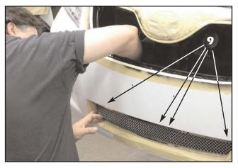
9. Use wide masking tape to tape up the lower grille opening. Carefully insert the lower mesh and frame into the factory lower grille opening and install a 1" O.D. by 1/8" I.D. black plastic washer onto each mounting stud and install an 8-32 ESNA half nut (as shown) and tighten (LE, Hybrid & XLE shown, SE installation procedure is the same).
