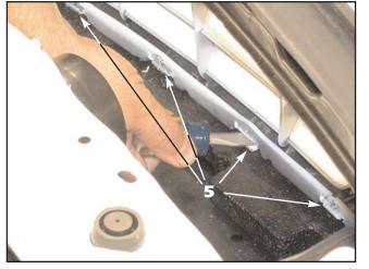
Use a wide flat blade screwdriver to pry on the factory grille mounting tabs. Pull out on the grille as you pry on the mounting tabs to release them.
