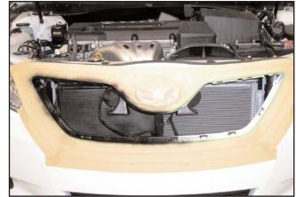
11. Use masking tape to tape around the factory grille opening 1/2" inside from the face of the bumper cover. Use flat or semi-gloss black paint and paint everything inside the taped factory grille opening that would be visible through the mesh grille, including across the top of the grille opening.
