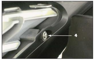
Remove the two mounting screws on the inside top of the grille (one each side at the top corners).
