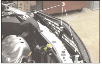
3. Lift straight up on the bumper cover and rest the bumper cover on the center support bracket. This will give you more working room for the following procedure.
