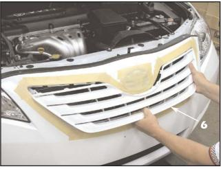
6. Continue pulling out on the grille until it completely unclips from the bumper cover.
