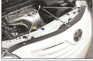
1. Open the hood and remove the outer phillips screws, center 10mm hex bolt and corresponding push fasteners to release the bumper cover from the support brackets.
