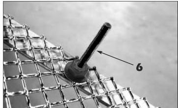
6. Prior to upper grille installation, apply black paint to the upper grille's lower studs and ESNA nuts to help conceal them once the grille is installed.
