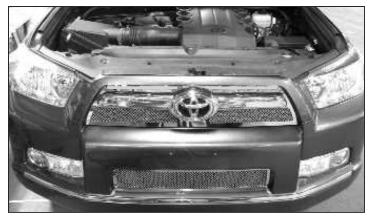
11. Reinstall the radiator support panel bracket back onto the vehicle. Peel off the protective coating from the upper and lower surrounds and use a mild solvent and a soft, clean cloth to remove any glue residue. Use alcohol or glass cleaner and a soft, clean cloth to remove any solvent residue.
