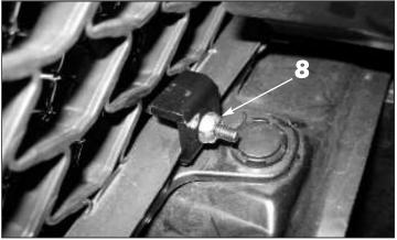
Install the supplied upper grille lower mounting brackets, part number 1073-0159-10 and secure them using the supplied #8-32 ESNA half nuts but do not tighten completely at this time.
