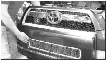
5. Once the masking tape has been removed, use a 9mm or 11/32" socket to tighten the #8-32 ESNA half nuts until the washers no longer rotate. Install the 3" long bracket onto the center bottom stud and the 4-1/2" long bracket onto the center upper stud and use the supplied #8-32 ESNA half nuts to secure. DO NOT OVERTIGHTEN the nuts or you could indent the stainless steel surround at the stud locations.
