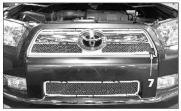
7. Peel back one corner of the protective coating on the lower stainless steel surround, then align the upper mesh grille into place making sure the studs pass throught the factory openings in the grille.
