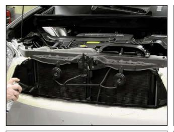
13. Use masking tape to tape around the factory grille even with the lower mounting holes drilled in the previous step. Use flat or semigloss black paint and paint everything inside the taped factory grille opening that will be visible through the mesh grille.
