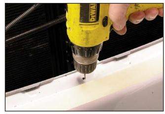
12. Use a 1/8" drill bit to drill through the marks made in the previous step. Make the holes into a slot by using the drill to connect the holes. This will allow for slight side to side adjustment when the grille is installed.
