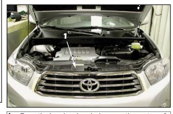
1. Open the hood and push down on the centers of the plastic push fasteners securing the radiator cover to release them. Remove radiator cover (save for reinstallation).
