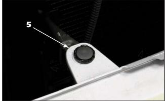
5. Reinstall the lower factory push pin at the bottom of the factory grille.
