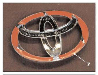
7. Clean the back of the emblem and install the supplied double faced tape (where shown).
