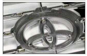
Carefully remove the emblem from the OEM grille by unclipping it.
