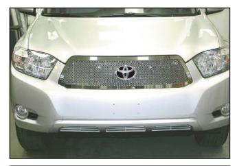
16. Close the hood and check for proper grille to hood alignment. You might have to loosen the side bolts and push the grille in if the edges are out beyond the hood's rubber seal.
