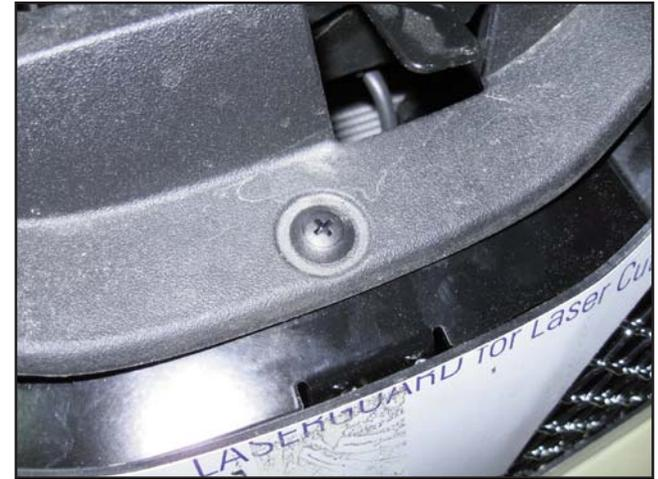
**14.** If the center factory push pin will not hold, install the E&G supplied push pin.
