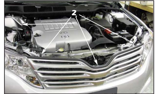
2. Remove the two (2) factory screws and the factory center push pin retaining the top of the factory grille.
