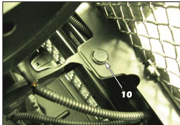
10. Align the mesh grille into the factory grille opening once all the protective masking tape is removed. Install the factory push pin removed in **Step 3** to hold the grille from moving during the factory bolt installation.
