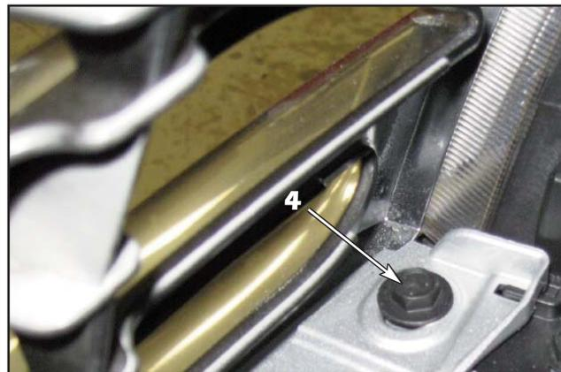
4. Remove the two (2) 10mm hex bolts (where shown, 1 each side), pulling the grille forward for bolt access.
