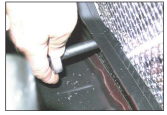
23. Install a small black plastic washer and a #8-32 ESNA half nut onto each of the lower four (4) mounting studs and tighten until the lower edge of the **mesh grille** is tight against the bumper cover.
