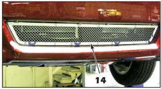
14. Align the lower mesh grille assembly into place, then reach through the upper grille opening to install the supplied small black plastic washer and a #8-32 ESNA half nut onto the center lower mounting stud. Tighten only until the washers no longer rotate but DO NOT OVERTIGHTEN. Overtightening will indent the surround at the stud location.
