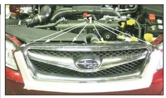
1. Open the hood and carefully apply several layers of masking tape to the painted upper and lower grille openings (around the upper factory grille). Remove the six (6) factory push fas tener across the top of the factory grille.
