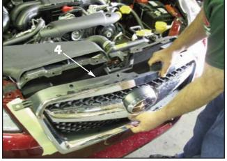
Once the bottom screws have been removed, pull the grille up and out to clear the bumper cover. The lower side alignment tabs may break off during the removal procedure.
