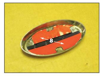
Remove the factory double faced tape and install the supplied .045" x 1" double faced tape (as shown), then remove the double faced tape liner (not shown).
