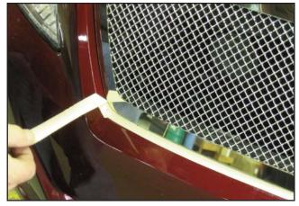
Peel off the protective masking tape from the bumper cover by pulling it back over itself to minimize breakage.
