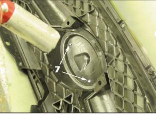
**6**. Use a heat gun to carefully heat the area behind the emblem to soften the factory double faced tape.
