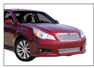
23. Peel off the protective cover from the stainless steel surrounds. Thoroughly clean the grilles to finish the installation. CAUTIONI Be careful while cleaning as the edges of the stainless steel can be very sharp.
