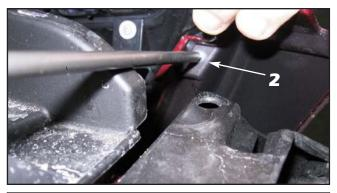
2. Remove the phillips screws that attch the factory grille to the bumper cover.
