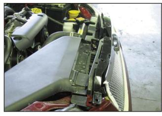
**23.** Reinstall the factory plastic panel removed in **Step 19**.
