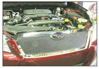
**22**. Install the factory plastic push fasteners to secure the E&G grille top plate to the support.
