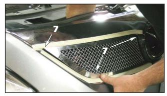
7. Tuck the surround outer corner underneath the factory grille surround and install the supplied large black plastic washer and #8-32 ESNA half nut onto the outer upper mounting stud. Tighten only until the grille section is snug. Install the large black plastic washers and #8-32 ESNA half nuts onto the outer lower stud (as shown) and the inner upper stud. Repeat procedure on the opposite side.
