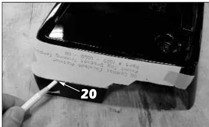
20. Cut out and align the front tag bracket trimming template (last page of this manual) and align it onto the sides of the front license plate bracket and mark the new edge you must cut to clear the mesh grille (trimming not shown at this time).
