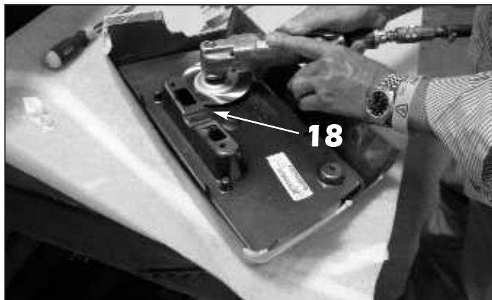
18. Trim the upper mounting boss from the inside of the front license plate holder.
