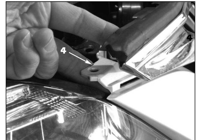
4. Once the outer screws are removed, pull up and forward on the factory grille to release the sides from the bumper cover.
