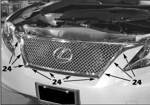
24. Align the assembled grille back into place, making sure that the factory mounting tabs pass back through the slots in the bumper cover.
