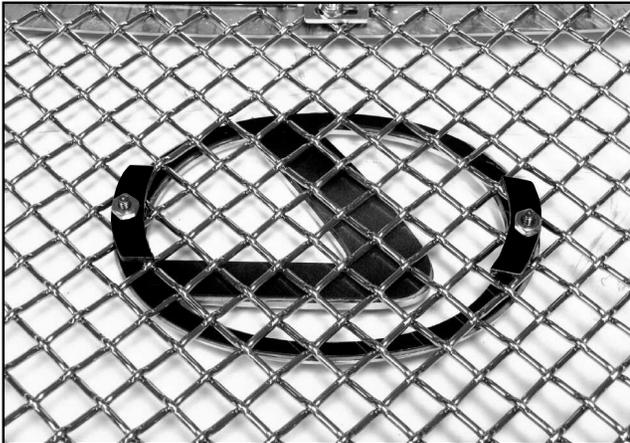
21. Install the emblem onto the mesh grille, making sure the emblem is perfectly centered top to bottom and left to right. Retain the emblem using the supplied mounting washers, #10 S.S. lock washers and the #8-32 hex nuts.
