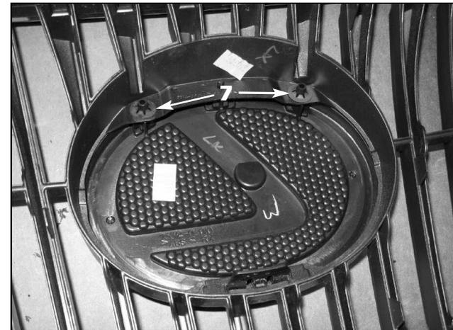
7. Use a small flat blade screwdriver to pry off the upper retaining clips, then remove the factory emblem from the grille.
