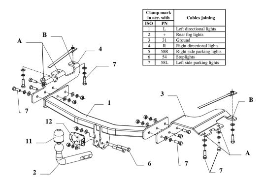
This towbar is designed to assembly in following cars: CHRYSLER VOYAGER and CHRYSLER GRAND VOYAGER both produced since 04.2001 till 03.2008 and is prepared to tow trailers max total weight 1600 kg and max vertical load 80 kg.
