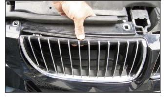
Pull forward on the top of the bumper cover and push up on the centers of the upper mounting tabs and push the grille sections forward to remove them from the bumper cover. *Note*: If the factory grille have chrome verticle bars, scuff the chrome verticle bars and paint them flat black.
