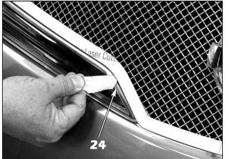
24. Once both mounting brackets are secured, lift up slightly on the grille and remove all protective masking tape from the front of the bumper cover and headlamp lenses.
