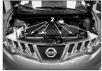
2. Remove the threaded plastic fasteners retaining the top of the factory grille.
