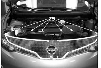
25. Reinstall the push fasteners removed in Step 2 to secure the top plate to the radiator support panel.
