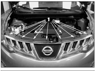
1. Open the hood and remove the push fasteners retaining the two plastic covers.
