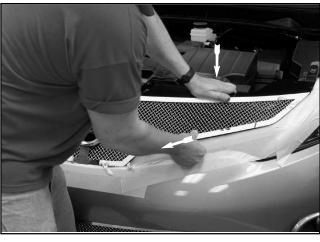
22. Pull the driver side of the grille slightly towards you and down until the mounting bracket lines up and begins to fit into the slot above the lense.
