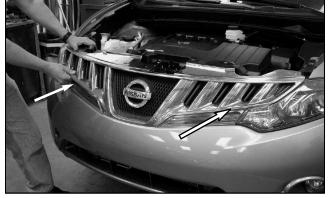
4. Pull the grille out so that the outer clips from the previous step clear the mouting slot, then lift up slightly on the grille in order to get your hand between the bottom of the grille and the top of the light (where shown). Give a quick pull straight out to release the next inboard mounting clips (one each side at arrow locations), the clips are not easily accessable with tools, so the mounting clips might break during removal but they are not reused.
