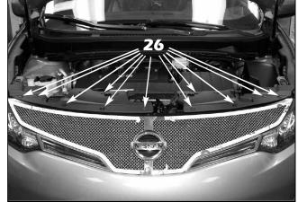
26. Reinstall the two factory plastics covers over the E&G top plate, reusing the factory push fasteners removed in Step 1.
