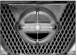
8. Unclip the factory emblem from the O.E. grille for installation onto the E&G Mesh grille.
