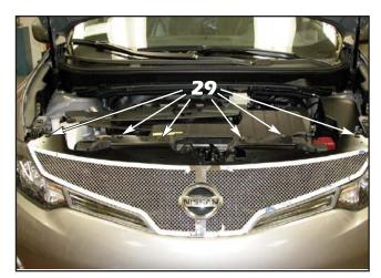
**29**. Reinstall the push fasteners removed in **Step 2** to secure the top plate to the radiator support panel.
