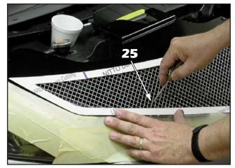
25. Pull out on the grille an push down until the mounting brackets line up with the mounting slot above the lense. Use a small flat blade screw driver to push down on the center of tab while pushing back onto the bottom of the grille until the tab clips into the mounting slot.
