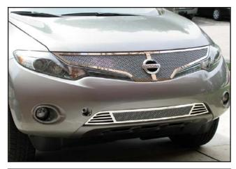
31. Remove the protective coverings from the grille sections and thoroughly clean the grille once you are finished the installation. A mild solvent followed by glass cleaner works very well. CAUTION! Be careful while cleaning the edges of the grille frame as the edges of the stainless steel can be very sharp.
