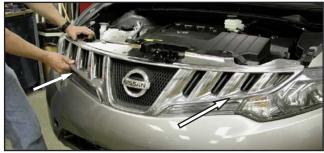
4. Pull the grille out so that the outer clips from the previous step clear the mouting slot, then lift up slightly on the grille in order to get your hand between the bottom of the grille and the top of the light (where shown). Give a quick pull straight out to release the next inboard mounting clips (one each side at arrow locations), the clips are not easily accessable with tools, so the mounting clips might break during removal but they are not reused.
