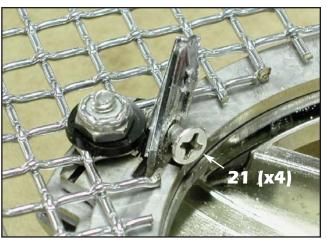
21. Turn the grille over and use a 3/32" drill bit to drill through all four (4) mounting tabs close to the surface of the grille and install the supplied #4 x 3/4" oval head phillips screws to secure the emblem to the mesh grille.
