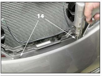
**14.** Use a 1/8" drill bit to drill through the marks made in the previous step, then use the drill to connect the holes making a mounting slot. This will allow for slight left to right adjustments during the grille installation.
