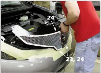
23. Remove any masking tape that could get caught underneath the center portion of the grille at the mounting pin locations.
