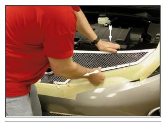
**26**. Pull the driver side of the grille slightly towards you and down until the mounting bracket lines up and begins to fit into the slot above the lense.
