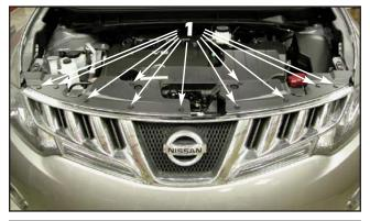
1. Open the hood and remove the push fasteners retaining the two plastic covers.
