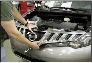
6. Using a flat blade screw driver, lift up on the center of the clips shown in Step 5 to release them when pulling the center of the grille free from the bumper cover.
