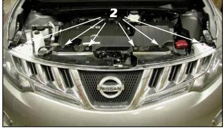
2. Remove the threaded plastic fasteners retaining the top of the factory grille.
