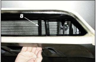
8. From underneath the vehicle, insert the lower grille mounting brackets between the metal bumper reinforcement and the styrofoam filler approximately 1" inside the outer veticle dividers (on each side). The tension of the angle the brackets rest against the metal bumper and the bumper cover will hold the brackets in place while you align the lower mesh grille into the opening.
