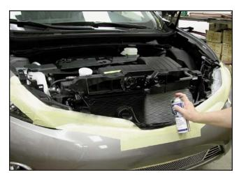
15. E&G recommends that everything visible in the grille opening be painted flat or semi gloss black. You will see through the E&G grille once it is installed and blacking out the radiator, bumper reinforcement, lower mounting holes on light colored vehicles, etc. will make for a professional appearing "factory" installation.
