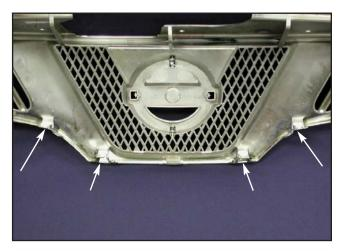
5. The photo above shows the locations of the four lower mounting clips. The grille is shown removed from the vehicle in order to show the locations as they are difficult to photograph with the grille still attached to the mounting brackets.
