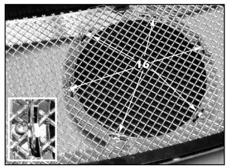
16. For "Ultimate" grilles using the mesh block off plate: Turn the grille over and install the supplied stainless steel emblem retainers using the #4-40 countersunk phillips screws (one per tab). Slide the retaining clips between the mesh and the emblem surround from the front side. Use a pointed tool to align the screw holes over the threaded holes.
