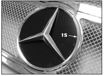
15. For "Ultimate" grilles using the mesh block off plate: Insert the factory emblem mounting tabs in the slots cut into the mesh block off plate and the emblem surround.
