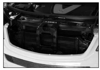
10. Once the lower slots are finished, use masking tape to tape up to the center of the slots and apply flat or semi-gloss black paint to everything inside the grille opening that would be visible through the mesh grille, including the top portion of the front bumper reinforcement.
