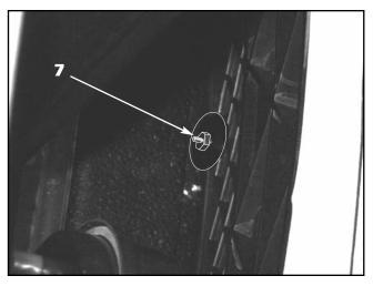
7. Carefully install the supplied black plastic washers and #8-32 ESNA half nuts onto each of the mounting studs and tighten. You might have to trim the washer to fit flush against the back of the factory grille. **DO NOT OVERTIGHTEN** or you could indent the grille surround at the stud locations.
