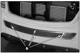
6. With the factory grille removed, align the lower mesh section to the back of the lower mesh surround and place it into the lower grille opening, making sure the four (4) mounting studs pass through the existing openings in the factory lower grille.
