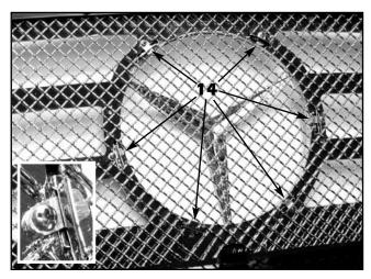
14. For "Ultimate" grilles not using the mesh block off plate: Insert the factory emblem mounting tabs in the slots cut into the emblem surround and install two (2) of the supplied stainless steel emblem retainers using the #4-40 countersunk phillips screws at all locations. It may be necessary to clip a wire or two for additional retainer clearance.
