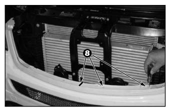
8. Measure and mark the center of the bumper cover grille opening. Cut out the supplied lower hole location template and align it with the driver side raised sections of the factory bumper cover and tape it into place to prevent it from shifting. Use an awl or pointed tool to mark the hole locations on the template onto the bumper cover. Flip the template over and mark the passenger side.
