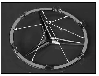
12. For Stainless Steel version: Apply the supplied double faced tape to the back of the emblems between the mounting tabs. Make sure the edges of the tape are not hanging past the edges of the emblem.
