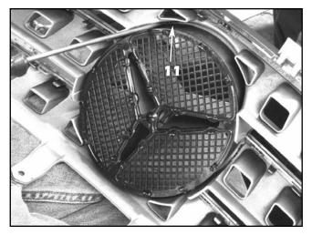
11. Use a small flat blade screwdriver to push on the mounting clips securing the factory emblem to the grille and remove the emblem.
