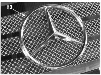
13. For Stainless Steel version: Peel off the protective tape from the face of the mesh grille surround and use a mild solvent to remove any tape residue. Follow with alcohol to remove any solvent residue.
