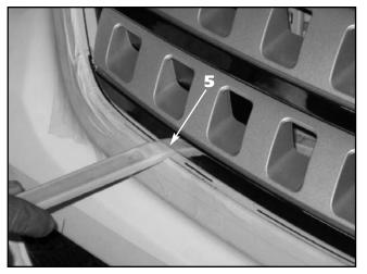
5. Use a plastic spreader or other non-metallic tool to press up from the outside of the grille where the mounting tabs are located and push the grille in to release the lower edge of the grille from the bumper cover, then remove the grille from the vehicle.
