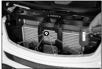
9. Use a .125" (1/8") drill bit to drill through the marks made in the previous step, then use the drill bit to connect the holes, making a small slot. This will allow for slight left to right adjustments when installing the mesh grille.
