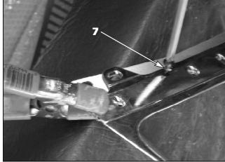
7. Attach the top plate to the chrome grille frame using the supplied 3/4" black truss head screws. The screws will go through the top of the factory chrome frame first, then through the E&G top plate underneath the factory grille frame. Screws must be installed from the top.
