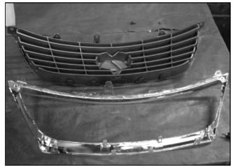
5. Unclip the grille insert from the chrome frame and remove it (not reused).
