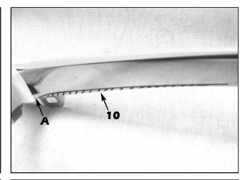
Align the curved edge of the grille trimming template with the inside top edge of the chrome surround. Use a grease pencil or sharpie to mark the chrome surround at the upper outer corners as shown (each side). This small area must be removed prior to the mesh grille installation. Blend into the sides of the grille (A).
