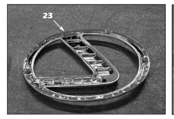
23. Remove the factory double faced tape from the back of the Lexus emblem. Using the supplied double faced tape, cut it into 1/8" wide strips and apply the tape to the outside edge of the emblem (as shown).
