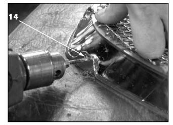
14. Use a 1/8" drill bit to create a small slot in the lower tabs located on the factory chrome frame. Make them wide enough for to install the .130" wide cable ties supplied with this kit.
