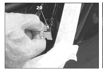
20. Carefully use a razor blade to trim the openings square with the edge of the opening and to remove any plastic shavings left from the drilling procedure.
