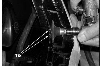
16. Use a small disc grinder to remove the two lower tabs on the left and right lower corners of the bumper cover to allow the assembled grille to fit without interference.
