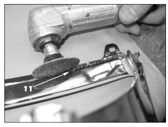
Use a small disc grinder to remove the small portion of the chrome grille surround marked in the previous step.
