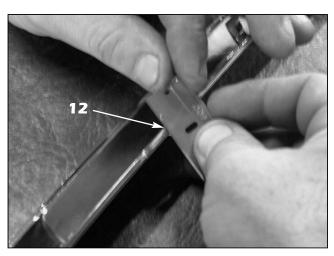
12. Inspect the inside edge of the factory chrome frame carefully. If there are any high spots or high edges from a rough casting, shave them down CAREFULLY with a razor blade or X-Acto knife. If you do not, the stainless steel frame on the mesh grille with not fit flush against the chrome frame.
