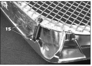
15. Install the blue TEFZEL cable ties (designed for harsh environments and high/low temperature conditions) through the slots made in the previous step and through the slots in the stainless steel frame. Orient the cable ties as shown in the above photo. Tighten until the stainless steel frame is firmly against the factory chrome frame, then trim off the excess cable ties.
