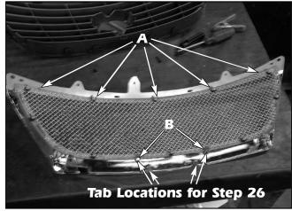
Align the mesh grille behind the factory chrome frame, making sure to hook the top edge behind the screws installed in Step 7 (A), then *carefully* pull the bottom of the factory chrome frame out until the two lower tabs (B) clear the stainless steel frame. Once clear, lower the stainless steel mesh frame into place.
