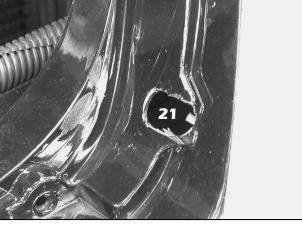
21. This is finished notch needed to clear the wire tie securing the mesh section tight against the factory chrome frame. Without this notch, you will not be able to install the grille.
