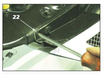
**22.** Install the supplied **#8 black truss head screws** to secure the E&G grille top plate to the core support.
