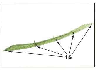
**16.** Align the lower mesh section over the back of the lower surround, then trim the ends from the preinstalled black cap plugs and push them down over the studs.
