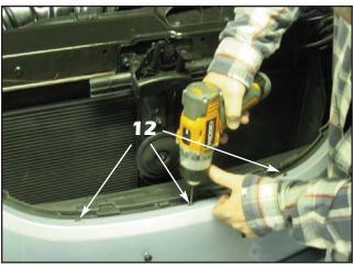
**12.** Remove the template and drill though the marks made in the previous step..
