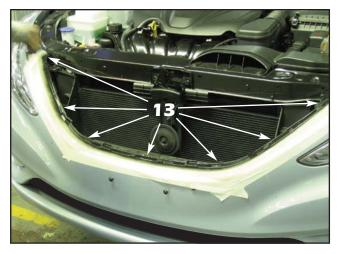
13. Use masking tape to tape up to the centers of the slots made in the previous step and scuff the paint on the bumper cover. Paint the return edge of the bumper cover and anything inside the grille opening with flat or semi-gloss black paint.
