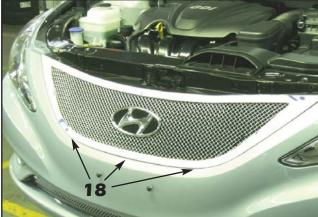
18. Remove any masking tape that could get caught between the grille and the bumper cover. Align the lower mounting pins into the slots drilled in Step 12 and push the upper mesh grille firmly into place.
