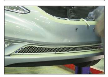
17. Align the lower mesh grille assembly into place, then reach through the upper grille opening to install the supplied large black plastic washers and #8-32 ESNA half nuts. Tighten only until the washers no longer rotate but DO NOT OVERTIGHTEN. Overtightening will indent the surround at the stud locations.
