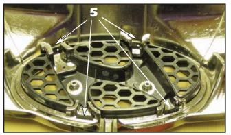
Use a small flat blade screwdriver to pry on to four (4) retaining clips and remove the emblem and backing from the factory grille.
