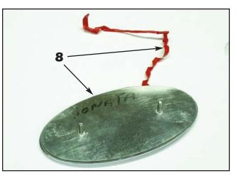
8. Install the supplied .045" x .250" double faced tape to the back of the emblem. Peel back a small corner of the double faced tape backing and align the emblem backing plate over the factory emblem. Once properly aligned, peel off the double faced tape liner and press the emblem firmly to the backing plate to set the tape.
