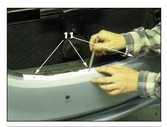
**10.** Measure and mark the exact center of the factory grille opening.
