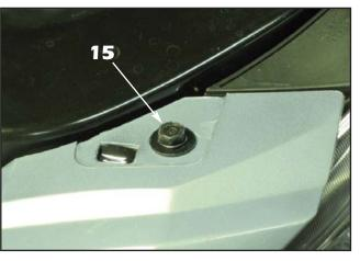
15. Reinstall the 10mm hex bolts removed in **Step 2**.
