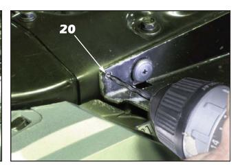
**21.** Use a .125" (1/8") drill bit to drill through the outer holes on the top mounting plate once the grille is level and centered.
