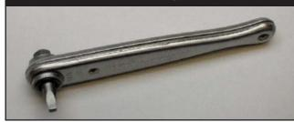
5. One way to remove the lower four (4) factory mounting screws is to use a small ratcheting screw driver or a ratching box wrench and a #2 square drive short bit (as shown). The large plastic screws that secure the bumper cover to the black bumper styrofoam need to be removed using a #3 square drive bit (not shown).
