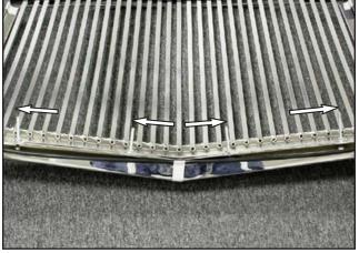
12. It may be necessary to bend the upper and side mounting studs to fit through the enlarged factory mounting holes. The studs should be slightly bent in the direction the arrows are shown in the above photo (studs bend towards the sides of the grille).
