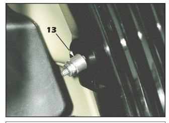
13. Once the mounting studs are passed through the enlarged factory mounting holes, install black plastic washers, #10 flat washers, #10 lock washers and 10-24 hex nuts across the top and tighten. Do not let the top studs hit the inside of the grille that could dimple the chrome plated metal (carriage bolt equipped grilles can not dimple the metal). The two side studs will require the additional use of the supplied 5/16" PVC spacers installed prior to the 8-32 ESNA half nuts.
