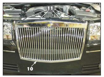
10. Once the paint is dry, align the Classic Grille's side mounting studs with the factory enlarged mounting holes in the bumper cover before you align the upper mounting studs with the enlarged factory mounting holes. If the studs do not line up with the enlarged factory holes, see the following stud alignment information.
