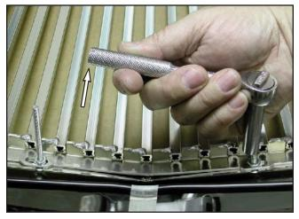
12. The best ways to bend the studs are with vise grips at the base of the studs (not shown) or with a deep socket that fits to the bottom of the stud and socket wrench to provide leverage for bending (shown). Bend slowly and carefully and test fit the grille to check your progress. Do not overbend the studs.
