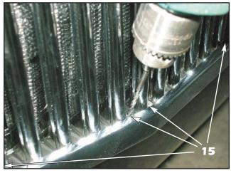
14. Push the lower part of the classic frame in while pushing out on the bottom of the bumper cover (if needed, use a wide flat blade screwdriver to pry the bottom of the bumper cover to meet the back of the grille frame).
