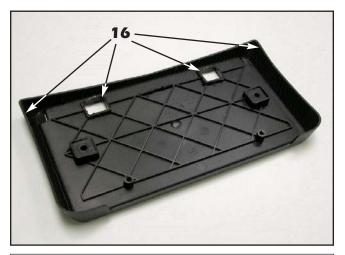
16. Trim the front tag bracket (if equipped), removing the top mounting bosses and trimming the left and right extensions that originally fit into the front grille opening recess. When finished, the modified tag bracket should look this this.
