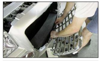
6. Remove the lower four (4) screws by pulling the grille out as far as you can for screw removal clearance. Remove the screws left to right, the subsequent screws will be easier to remove as you will be able to pull the grille farther out. **Removal tip:** If you can not access the lower screws, pull the factory grille out and straight up, the lower four screws will simply pull through the urethane bumper cover (the lower holes are not reused).
