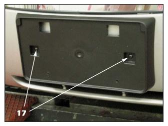
Align the modified front tag bracket below the mesh grille (where shown). Install the modified tag bracket back onto the bumper cover by drilling new 3/32" mounting holes and reusing the factory screws (DO NOT OVERTIGHTEN). Reinstall the radiator support panel cover (not shown).
