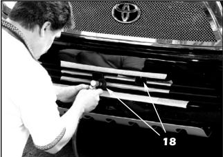
18. Use a small grinded to remove the plastic bosses. Grind them until they are flush with the grille fins along the sides and bottom, and across the top until you make contact with the J-clips securing the front bumper cover.
