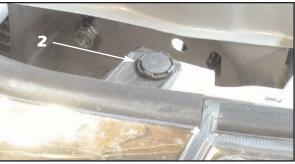
Remove the two factory push pins retaining the sides of the factory grille.
