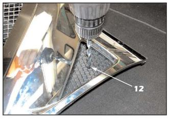
12. Drill a 1/4" hole throught the center of the small left and right grille recesses (where shown). Enlarge the hole as needed until the studed grille fillers fit into the left and right grille recesses.
