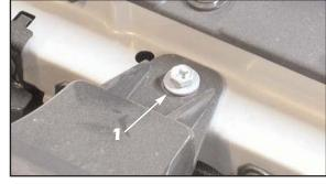
Open the hood and remove the two factory 10mm hex bolts retaining the center of the grille.
