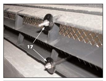
17. Install a black plastic washer and a #8-32 ESNA half nut onto each stud and tighten. Do not overtighten or you will indent the stainless grille surround at the stud locationsl
