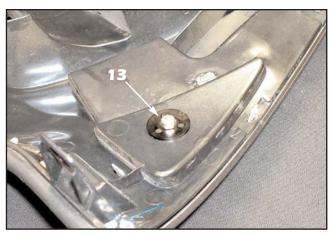
Turn the upper grille over and install a black plastic washer and an ESNA nut onto the protruding studs and tighten.
