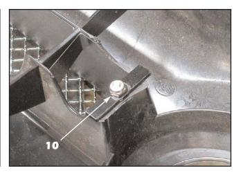
Install the rectangular retainers onto the studs mounted on the emblem surround and install a #8-32 ESNA half nut onto each stud and tighten, making sure the emblem surround does not shift.
