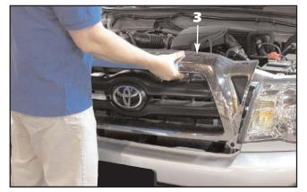
**3**. Lift straight up on the grille to release the lower clips located on the left and right sides of the factory grille.
