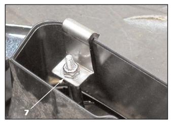
Turn the grille over and align the mounting brackets over the eight (8) studs welded to the grille frame and install the supplied #8-32 ESNA half nuts. Snug the grille but do not tighten at this time. Leave the grille loose until you remove the protective masking tape installed in Step 4.
