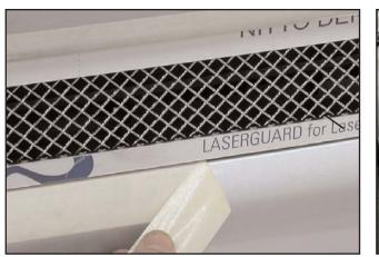
18. Carefully remove the masking tape by pulling it back over onto itself to minimize the chance that the tape might break. If the tape looks like it will get caught, lift up or move the grille frame from side to side for additional frame clearance.
