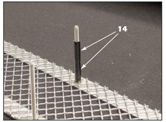
14. Trim the ends from the supplied vinyl caps and install two (2) onto the bottom center and side studs. It is not necessary to install the vinyl caps onto the top stud.
