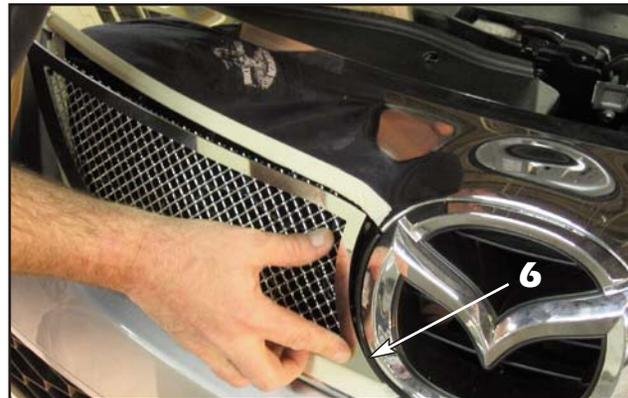
4. Align the mesh sections over the surrounds and trim the ends from the supplied #8-32 black cap plugs and install them over the mounting studs.
