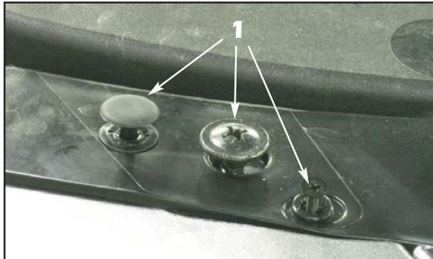
1. Remove the factory mounting hardware from the bumper cover where it attaches to the core support.
