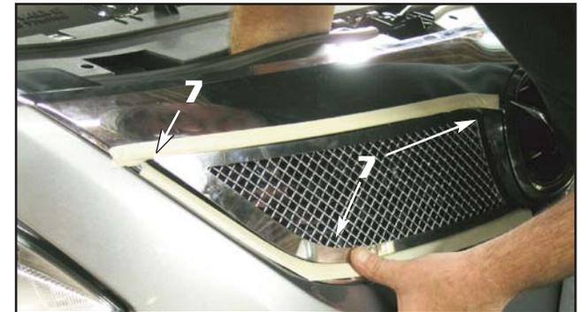
7. Tuck the surround outer corner underneath the factory grille surround and install the supplied large black plastic washer and #8-32 ESNA half nut onto the outer upper mounting stud. Tighten only until the grille section is snug. Install the large black plastic washers and #8-32 ESNA half nuts onto the outer lower stud (as shown) and the inner upper stud. Repeat procedure on the opposite side.
