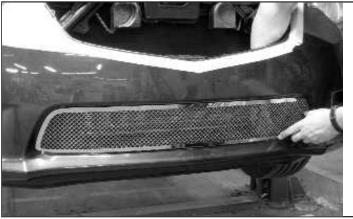
Install the lower mesh grille into the bumper cover and secure it using the supplied large black plastic washers and #8-32 ESNA half nuts. Tighten until the washers no longer rotate.
