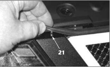
Reinstall the factory weatherstrip to the bumper cover.
