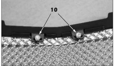
10. Once the weatherstrip is aligned, carefully install the top mount ing plate onto the upper mesh grille assembly, masking sure the weatherstrip does not shift. Install the supplied #8-32 ESNA half nuts to secure the top mounting plate. Start at the center and work your way out to the sides.
