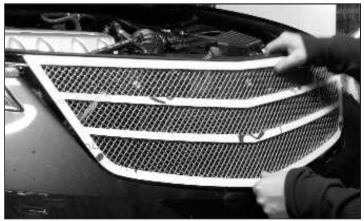
14. Once the paint has dried, align the lower mounting pins on the assembled mesh grille with the slots made in the previous steps and push the mounting pins into the slots until the grille is flush with the bumper cover.
