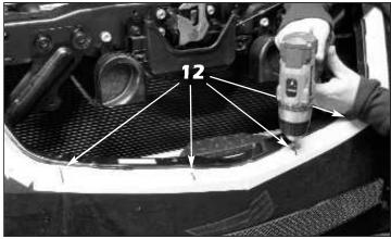
12. Use a 1/8' (.125") drill bit to drill through the marks made in the previous step. Use the drill bit to connect the holes, making small slots to allow for slight left to right grille adjustment.
