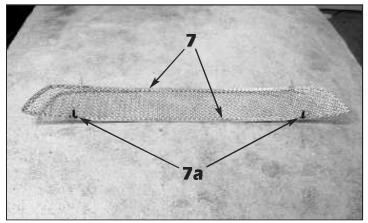
Install the supplied .045" x .250" double faced tape across the top and bottom portions of the lower mesh surround and align the mesh section into place and press it firmly to set the tape.
