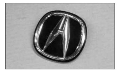
15. For customers who require the factory emblem installation: Install the supplied .045" x .250" double faced tape to back of the factory emblem and install it onto the supplied emblem mounting plate.
