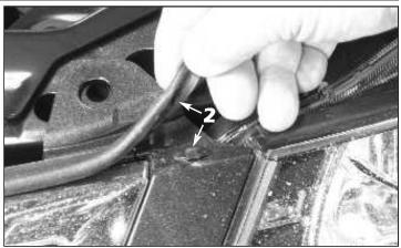
2. Pull the edges of the factory grille weatherstrip free from the mounting clips (one per side).
