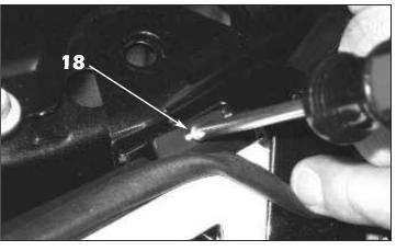
18. Once the mesh grille is level and perfectly centered, install the supplied #4 x 3/4" oval head phillips screws into the upper outer mounting tabs to secure the top edges of the grille to the bumper cover (one each side). Allow the screws to self tap into the bumper cover. *Paint the screw heads black to conseal them.*
