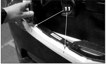
11. Cut out the supplied hole location template and use masking tape to secure it to the bumper cover once it is centered. Use an awl or similar pointed tool to mark the hole locations onto the bumper cover, untape the template, flip it over, tape it into place and mark the holes on the opposite side.
