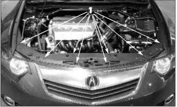
Open the hood and remove the eight (8) factory push pins securing the radiator support panel cover to the vehicle and remove it. Lift up on the centers of the push pins to release them.
