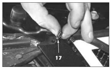
17. Use long nose pliers to squeeze the factory weatherstrip mounting pins and remove them from the bumper cover.17a. Reinstall the pins back into the factory weatherstrip.
