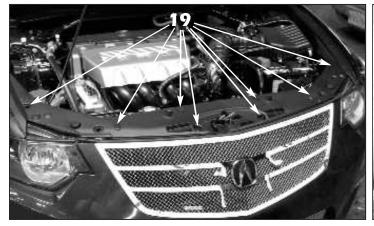
19. Reinstall the factory radiator support panel reusing the factory push fasteners.
