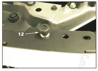
12. Install the upper factory bolts (removed in Step 2) through the upper mounting plate and into the upper grille mounting brackets. Make sure that the grille surround is slightly behind the edge of the hood by carefully lowering and closing the hood. Adjust in or out as needed. Hood adjustments can be made at the core support mounted rubber bumpers by threading them in or out. Once properly aligned, tighten the screws.
