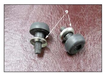
9. Install the supplied stainless steel washers onto the factory bolts that secure the top of the grille.
