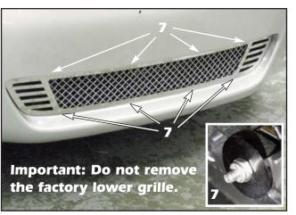
7. Apply protective masking tape around the factory grille opening (not shown). Align the mesh section and surround into the lower grille opening and install a large black plastic washer and a #8-32 ESNA lock nut onto the lower studs and tighten. Do not overtighten or you will indent the stainless grille surround at the stud locations! Once the hardware is tight, remove the masking tape.
