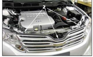
Remove the two (2) factory screws and the factory center push pin retaining the top of the factory grille.
