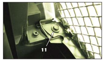
11. Align the factory shouldered bolts through the slots in the lower mounting plate and into the factory holes in the bumper cover and once the grille is perfectly centered, completely tighten the bolts.
