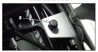
3. Use a flat blade screw driver to lift up on the center of the factory push pin located at the bottom center of the factory grille and remove the push pin.
