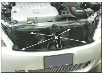
8. Apply protective masking tape to the bumper cover 1/16" infront of the small raised bumps across the top edge (under the factory grille) and the face of the headlights. Carefully paint anything inside the grille opening with flat or semi-gloss black paint that would be visible through the mesh grille, including the radiator and A/C condensor.
