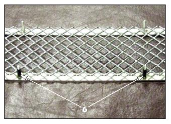
6. Prior to lower grille installation, trim the closed ends from the supplied vinyl caps and install them onto the center two (2) lower mounting studs.
