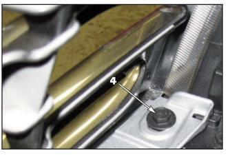
Remove the two (2) 10mm hex bolts (where shown, 1 each side), pulling the grille forward for bolt access.
