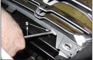
5. Remove the upper grille by inserting a flat blade screw driver under the lower mounting tabs and lifting up to release the tabs across the bottom edge of the grille. Start at one side and pull forward on the grille as the clips release.
