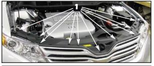
1. Open the hood and remove the factory push pins retaining the black radiator support panel cover and remove the cover. The large push pins are removed by lifting up on the center until the pin gets loose, then pull straight up to remove. The small push pins with the small center pin needs to have the center pin depressed, releasing the pin then lift straight up to remove.
