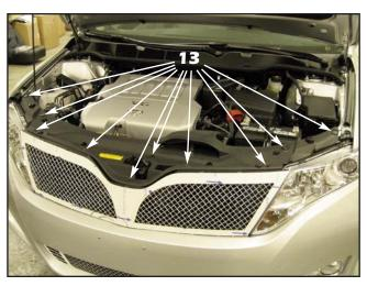
Reinstall the radiator support panel cover (removed in Step 1) using the factory push pins in the locations they came out of.
