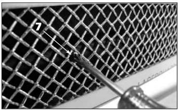
**7**. Install the supplied #4 x 3/4" oval head screws (paint the screw heads with black paint to help conceal them). Use an awl or similar pointed tool to make an impression to start the screw installation. Once the lower grille is secured, remove the protective masking tape (not shown).
