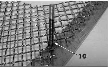
**10**. Paint the lower four (4) mounting studs on the upper grille assembly black prior to upper grille installation.
