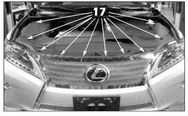
**17.** Reinstall the engine bay panels removed in **Step 1** and close the hood and lower the vehicle to finish the installation.
