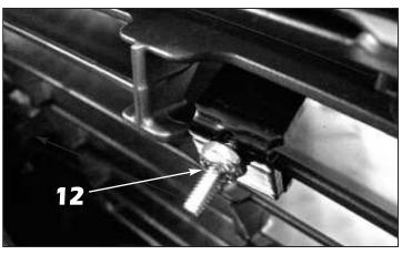
**12.** Install the supplied upper mesh retaining brackets onto the upper center four (4) mounting studs and install a #8-32 ESNA half nut. *Do not completely tighen at this time.*
