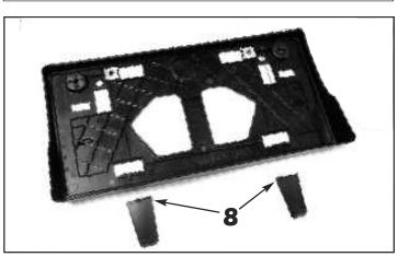
**8.** For vehicles equipped with a front license plate bracket: Remove the lower mounting tabs from the front license plate bracket.
