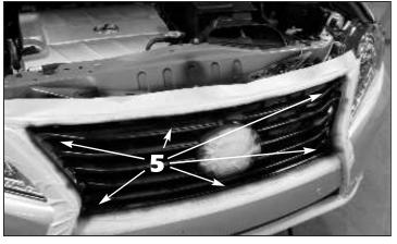
**5.** Apply flat or semi-gloss black paint to the factory grille insert and install the lower grille while the paint cures.
