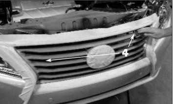
**4.** Carefully use a scotch brite pad or fine sandpaper to scuff the factory grille insert for the following paint procedure.
