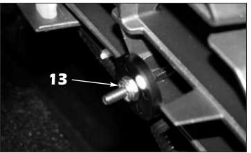
13. Install the supplied large black plastic washers onto the lower four (4) mounting studs and the top outer mounting studs. Install #8-32 ESNA half nuts onto each mounting stud. *Do not completely tighen at this time.*
