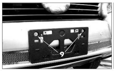
9. Remove the protective tape from the lower grille surround and use solvent and a soft, clean cloth to remove any glue residue. Use glass cleaner and a soft, clean cloth to remove any solvent residue. Reinstall the factory license plate bracket back onto the bumper cover, reusing the factory hardware.
