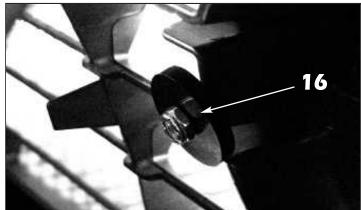
**16.** Install the supplied large black plastic washers onto the mounting studs and install a #8-32 ESNA half nut, Make sure the grille and emblem surrounds are in their proper postion and tighten the ESNA half nuts until the washers no longer rotate and the retainers are snug. **DO NOT OVERTIGHTEN** or you will indent the surround at the stud locations.
