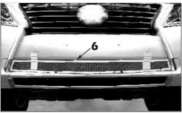
6. Align the lower mesh grille assembly into place, making sure it is perfectly centered. Use wide masking tape to hold it into place during the following screw installation procedure.
