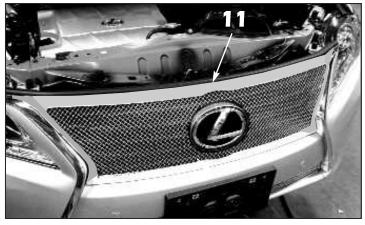
**11.** Remove any masking tape that could get caught underneath the upper mesh grille once it is installed. Carefully align the upper mesh grille assembly into place, making sure it is perfectly centered in the factory chrome surround.
