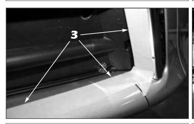
**3**. Close-up of the lower grille masking tape application. Match the arch of the lower grille center bar onto the painted bumper cover.
