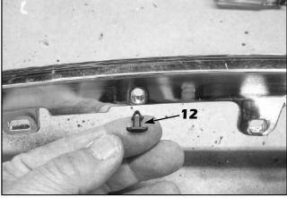
Make sure you remove all remaining small clips that hold the rubber weatherstrip to the top of the chrome surround (save for reinstallation).
