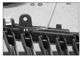
11. Use a small flat blade screwdriver to release the mount-
