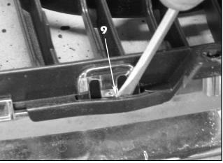
Using a small flat blad screwdriver, begin prying the insert away from the tabs securing it to the chrome surround across the bottom edge.
