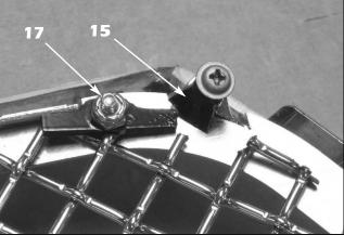
15. Use a phillips screw driver and the factory screws to attach the supplied mounting tabs onto the outer screw bosses (as shown).
