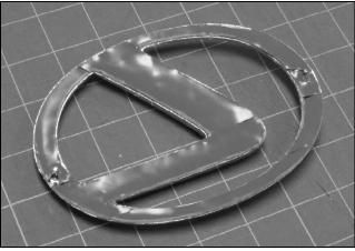
19. Install the supplied double faced tape to the back of the Lexus emblem as shown.
