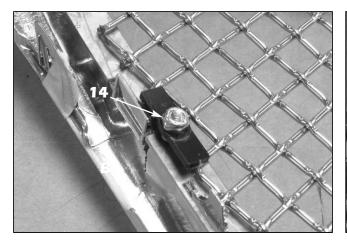
14. Install the supplied rectangular mesh retainers over the mesh section and install the supplied #8-32 ESNA half nuts to secure.
