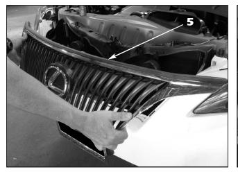
Across the bottom edge, push on the centers of the grille mounting tabs locking the factory grille to the bumper cover, then pull the grille straight out to remove.
