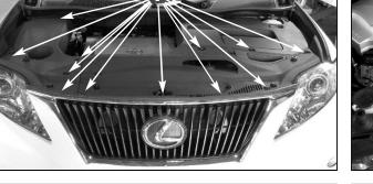
1. Open the hood and remove the push pins retaining the engine bay covers, then remove the covers.
