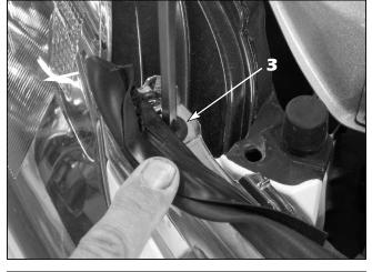
3. Pull forward on the factory weatherstrip and remove the outer retaining screws (one each side).
