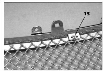
13. Align the mesh grille surround, mesh section and top plate behind the factory chrome surround, making sure the upper tabs line up with ones on the factory surround and the factory tabs on the sides and bottom pass through the slots in the E&G surround. Install (5) #8-32 ESNA half nuts across the top to retain the upper section of the mesh grille.
