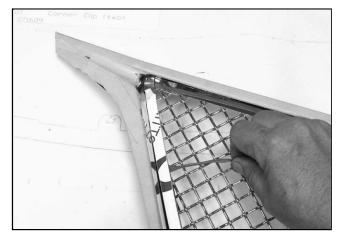
23. Peel back a small section of the double faced tape backing from each end of the overlay. Carefully align the overlay tightly against the factory chrome surround but do not scratch the chrome. Once the overlay is in place, pull off the lining from the double faced tape and press the overlay firmly into place to set the tape.
