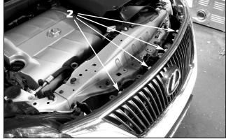
Remove the factory 10mm hardware retaining the top of the factory grille to the support.
