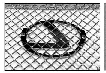
21. Install the emblem onto the mesh grille, making sure the emblem is perfectly centered top to bottom and left to right. Retain the emblem using the supplied mounting washers, #10 S.S. lock washers and the #8-32 hex nuts.
