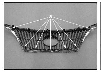
8. The factory grille insert is now ready to be seperated from the factory chrome surround. First remove all phillips screws holding the insert to the surround.
