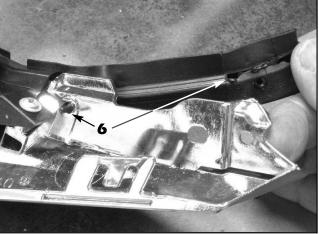
6. Once the grille is place onto a clean work bench, remove the upper weatherstrip and retaining clips (to be reused) by squeezing the bottoms of the retaining clips together before pushing them out of the mounting holes.
