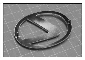
20. Peel off the tape backing and install the emblem backing plate with studs. Once the plate is attached, break off the factory emblem alignment pins as they could prevent the emblem from being properly centered on the mesh section.
