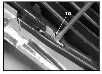
10. Use a small flat blade screwdriver to release the clips on the sides of the surround.
