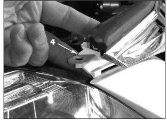
4. Once the outer screws are removed, pull up and forward on the factory grille to release the sides from the bumper cover.
