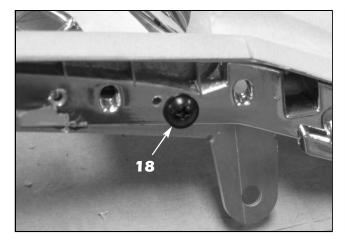
18. With the E&G surround pressed tightly against the factory chrome surround, drill a 7/64" hole through the center and the outer holes in the top plate and through the factory chrome surround. Flip the assembly over and install the supplied #8 x 1/2" black phillips truss head screws into the upper three (3) mounting holes from the top (outer hole shown). Do not install the screw up from the bottom.
