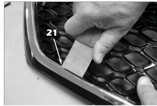
**21.** Turn the grille over and use a flat blade screwdriv er to push out on the upper hortizontal chrome moulding laignmeth tabs (not shown). Carefully use a tucking tool to slice through any double faced tape holding the chrome moulding onto the grille, then remove the chrome moulding.
