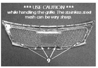
Carefully align the **upper mesh section** behind the factory chrome surround, making sure that the mesh section overhangs the surround opening the full perimeter. Make sure the mesh is tight against the lower alignment tabs (see arrows).
