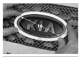
16. Install the emblem surround, making sure it is perfectly aligned. You may have to slightly slot the holes up and down in order for the surround to fit properly.
