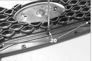
**20**. Turn the grille over and remove the fourteen (14) factory phillips screws retaining the factory chrome trim.
