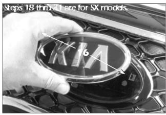
**18**. Remove the factory KIA emblem by using a flat blade screwdriver to unclip the emblem and pull it straight out.
