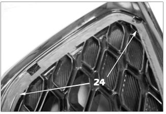
24. Additional grinding is necessary bewteen the arrows in the above photo. Hold the disc grinder at the same angle as the factory grille mesh and grind into the area underneath the factory chrome moulding until it is flush in height with the factory mesh. Approx. 1/8" of plastic needs to be removed from the sides of the factory grille.
