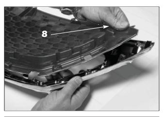
**B**. Remove the factory grille insert from the chrome surround by lifting it out.
