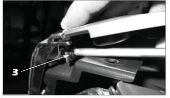
3. Pull the top of the grille out just enough to access the upper out top plate securing screws. Use a phillips screwdriver to remove these screws (one each end). Do not pull too far, you could damage the factory grille.
