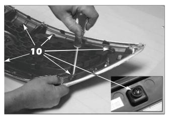
10. Once the mesh section is in place, realign the factory grille insert and install the supplied #8 x 5/8" stainless steel screws and stainless steel finishing washers. Do not let the mesh insert shift while aligning the factory insert. Make sure all factory tabs are aligned back into the slots in the factory insert.
