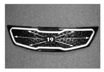
**19.** Apply masking tape to the chrome moulding on the factory grille.
