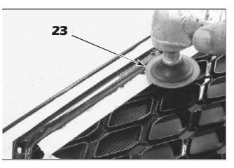
**23.** Extreme caution: Use a disc grinder to remove the raised portion of the factory grille around the factory grille mesh section. Grind the raised area until it is flush with the portion of the grille that was covered by the chrome trim.
