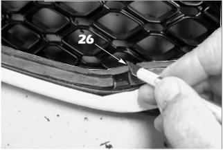
**26.** Once the mesh has been test fitted and it is flush, use an X-acto knife or a razor blade and remove any ground off plastic burrs prior to mesh installation.
