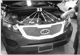
33. Reinstall all attaching hardware removed in Steps 1 through 4, then remove any remaining masking tape.
