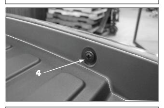
**4**. Remove the phillips screws securing the factory upper plate to the top edge of the grille and remove the top plate.
