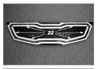
22. Apply masking tape to the grille recessed area and the surface around the chrome moulding recess.
