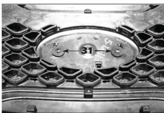
31. Align the factory emblem through the mesh section and the factory grille, then install the supplied 7/8° O.D. x 1/4° I.D. black plastic washers (two per boss) and the supplied #8 x 3/8° black truss head screws and tighten until the emblem is tight. You might need to trim the washers in order for them to lay flat against the back of the grille.
