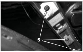
5. Pull the grille our far enough to expose the factory screws retaining the grille to the bumper cover. Remove these screws frist, then remove the screws across the bottom of the grille. Pull forward on the grille to remove it from the bumper cover.
