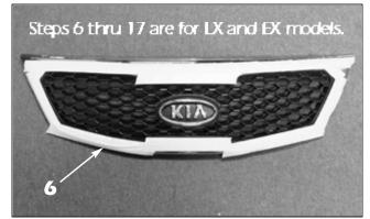
**6.** Place the factory grille onto a clean work surface and apply masking tape to protect the chrome finish of the surround.
