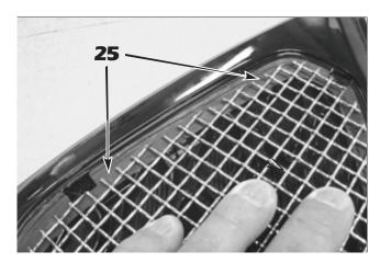
**25**. Align the **mesh section** over the factory grille and make sure that the mesh fits flush with the outer edge of the factory grille where the chrome moulding aligns. If the mesh is not flush, the chrome moulding will not fit properly when reinstalled.
