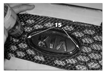
**15**. Use a 5/16" drill bit to enlarge the holes drilled in the previous step.
