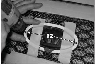
11. Align the supplied 22 gage hole drilling template around the factory emblem and once perfectly centered, use masking tape to hold it in place during the following hole drilling procedure.
