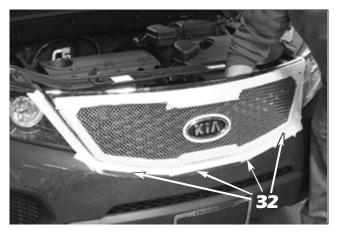
**32**. Reinstall the lower and side factory mounting screws (removed in **Step 5**) once the assembled grille is aligned with the bumper cover.
