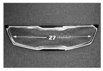
**27**. Align the **mesh section** and the factory chrome moulding over the factory grille.
