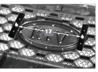
17. Install 3 hole mounting brackets and #8-32 ESNA half nuts onto the emblem ring studs and tighten.
